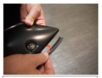
**STEP 9:** Attach the included rubber seal to the Fender Flares. Peel back 2" of the adhesive backing and position on the Fender Flare. Attach the seal to the Fender Flare, peeling back a few inches at a time. Attach rubber seal along all areas the Fender Flare will make contact with the vehicle body.
