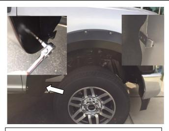
**STEP 7:** Loosely reinstall the lowest rear 7/32 in socket head screws through slot in the Fender Flare to the vehicle. Make sure the screws are securely engaged to the vehicle fender. Install provided Long Attachment Clips in remaining four (4) Fender Flare Slots. Loosely reinstall remaining 7/32 in socket head screws. Ensure part is still in the position of best fit and extrusion is in correct position before hand tightening all screws.
