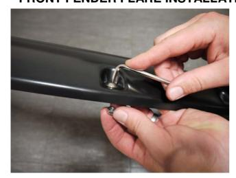
**STEP 1:** Attach the bolts to each Fender Flare using a 3/16" Allen key and a 10.0mm wrench/socket. (wrench/socket and Allen key not supplied). Ensure inside of Fender Flares where the rubber seal is attached is clean, using the alcohol wipes provided. Wipe away any residue with a dry clean cloth.
