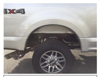
**STEP 10:** Clean the body areas where the Fender Flares will makes contact. Use the supplied alcohol wipe. A light misting on fender using a soap and water solution can aid in proper rubber placement
