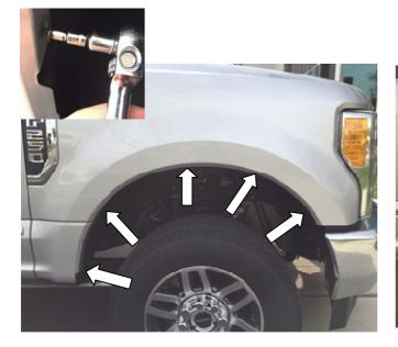
**STEP 5:** Remove all 5 7/32 in socket head screws and retain for installation of Fender Flares.
