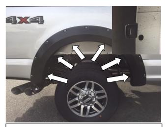
**STEP 11:** Place the Fender Flare onto the vehicle and fit into the correct position following the contours of the body. Use the twelve (12) provided "U" Shaped Retention Clips (six 6 per side) to secure the Fender Flare to the body. Make sure the dimple in the clip securely attaches in the slot on the Fender Flare.
