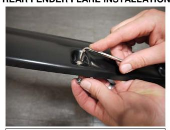
**STEP 8:** Attach bolts to each Fender Flare using a 3/16" Allen key and a 10.0mm wrench/socket. (wrench/socket and Allen key not supplied). Ensure inside of Fender Flares where the rubber seal is attached is clean, using the alcohol wipes provided. Wipe away any residue with a dry clean cloth.
