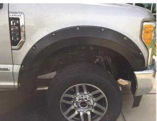
**STEP 6:** Place the Fender Flare onto the vehicle and fit into the correct position following the contours of the body. Ensure the slots in the part align with the holes in the fender from the previously removed 7/32 in socket head screws.
