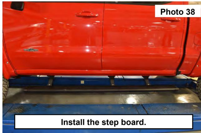
42. Slide the mounting block under each of the (3) mounts, then secure the step board using (2) of the supplied 6mm socket head bolts and (2) 6mm lock washers in each step mount. **See Photo 39.**
