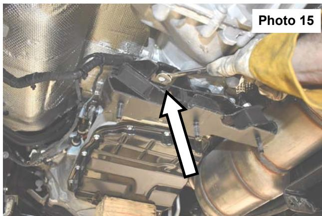
26. Using a 15mm socket, remove the (2) front transfer case crossmember mount bolts and remove the mount. Retain hardware. **See Photo 16.**
