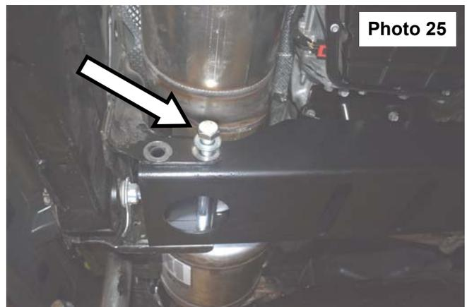
36. Torque to 120ft/lbs using 24mm socket and wrench. **See Photo 26.**
