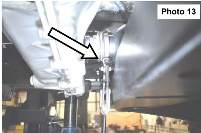
23. Using snap ring pliers, spread the snap ring and slide the driveshaft towards the front of the truck. **See Photo 14.**
