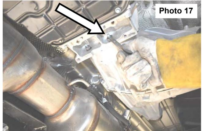
29. Carefully remove the transfer case from the truck.
