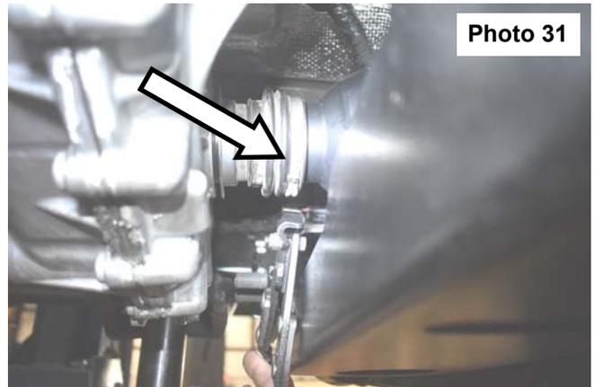
43. Attach the front driveshaft to the pinion flange using the factory hardware. Torque to 45ft/lbs using a 15mm socket.
