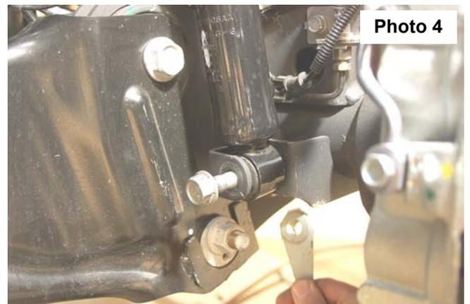
11. Lower the axle and remove the coil springs. Note there is a rubber push pin made on to the factory coil isolator to align the coil spring. Push on the top the pin to release the isolator from the frame coil pocket.
