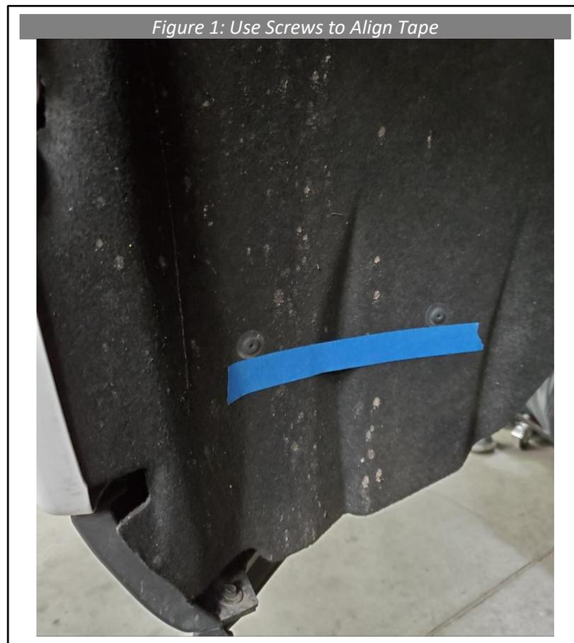
3. Look from below the truck to make sure there is nothing else behind this section of fender liner which could be accidentally cut.
