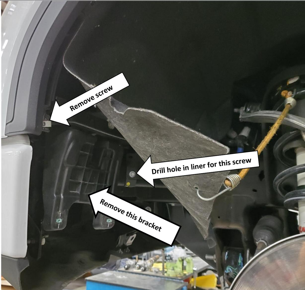
8. Return the fender liner to its original factory position. Drill a small hole in it so the screw shown in figure 12 can be used to hold it down.
