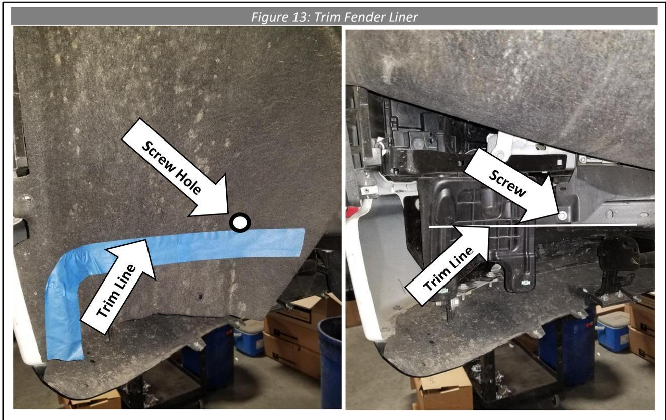
10. Using a sharp box cutter, poke thru the fender liner material and make the cut. Be very careful to not cut yourself or slip and cut into the paint. Return the fender liner to the factory position and reinstall all screws.
