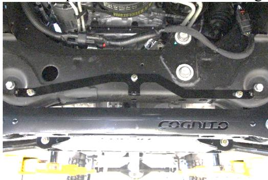
**Figure 3: Bolt bracket to frame**
