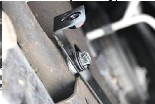
**Figure 4: Space bracket using (3) 5/16 washers**
