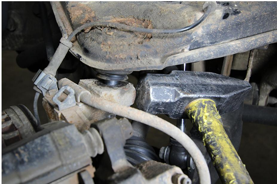
4. Remove the factory bolts and eccentric washers that connect the control arm to the frame and retain them for future use. Place them aside in order, so that they may be re-installed in the same manner they came off. The plastic inserts will need to be removed and discarded from the eccentric washers.
