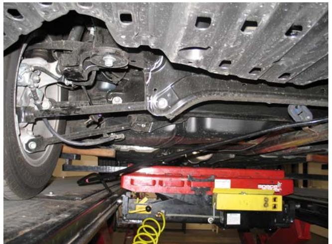
9. Your new Suspension Techniques swaybar comes with new Teflon lined bushings. You will be using the original equipment end links and bushing brackets. Install the new bushings onto the Suspension Techniques swaybar prior to installation.
