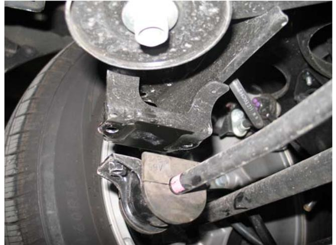
8. To remove the original equipment swaybar you must first remove the driver's side, then turn the swaybar towards the front of the vehicle and rotate the swaybar to remove it from the passenger side.
