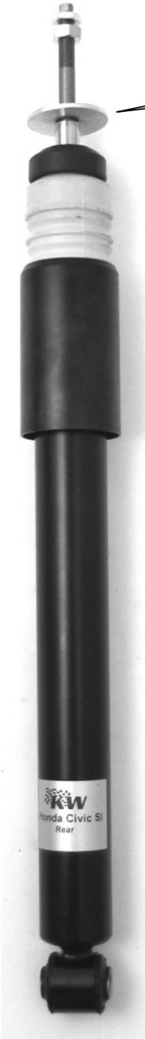
Tightening torque for the piston rod nut is 20 Nm (15 ft-lb). The damper unit has to be installed according to manufacturers recommended settings regarding tightening torque and fixing specifications.
