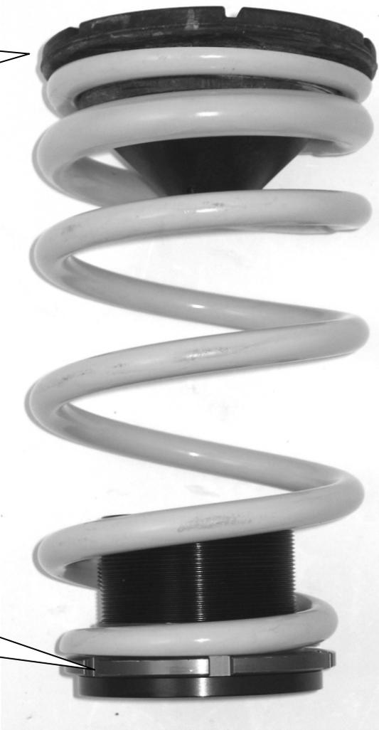
Mount the supplied height adjuster without rubber support between the body and the bottom end of the spring.
