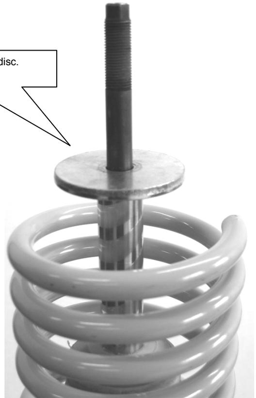
Install the factory supporting bearing and fix it with the supplied nuts. Tightening torque for the piston rod nut is 20 Nm (15 ft-lb). The strut unit has to be installed according to manufacturers recommended settings regarding tightening torque and fixing specifications.
