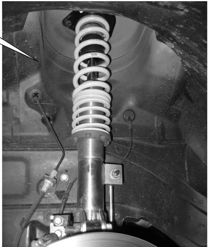
After you have completed installation of the suspension, check the clearance of the tyres to the front suspension strut. The minimum clearance at the narrowest point is 4 mm and must, where necessary, be provided using commercially available, Technical Inspectorate (German TUEV) approved spacers.
