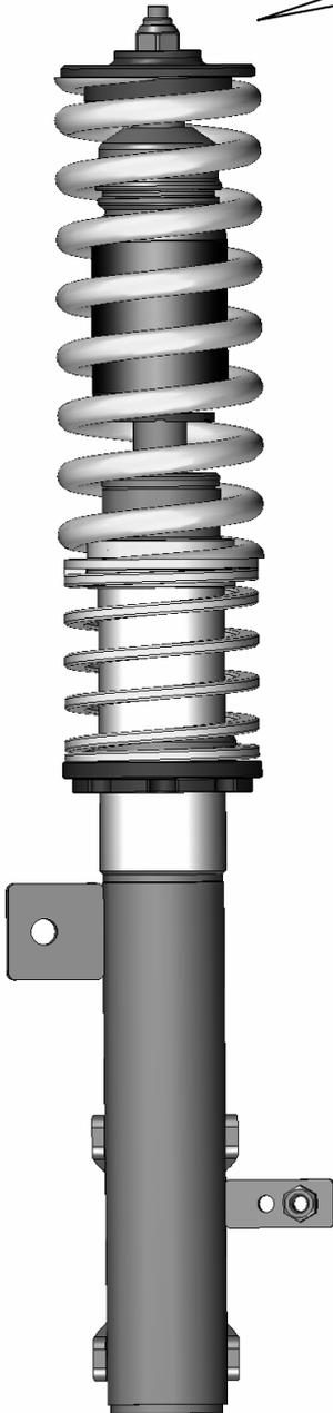
Install the factory supporting bearing and fix it with the supplied stop nut. Tightening torque for the piston rod nut is 35 Nm (26 ft-lb). The strut unit has to be installed according to manufacturers recommended settings regarding tightening torque and fixing specifications.
