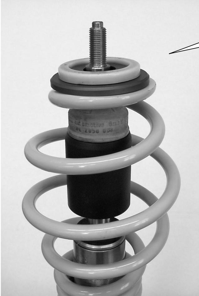
Supplied complete front coilover strut with supplied original axial bearing.
