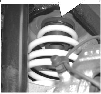
Unless there is no spring (Elastomer) supplied by the factory spring (Elastomer) has to be used. The factory spring (Elastomer) has to be in a good condition, otherwise it has to be replaced. Therefore only use spare parts for BMW E46 M-technic. Tightening torque for piston rod nut is 25 Nm (18 ft-lb). The rear axle shock absorber has to be installed according to the car manufacturers installation instructions.
