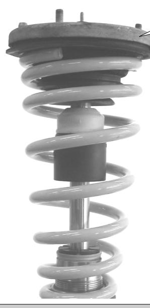
Attach the original supporting bearing with all necessary parts to the strut using the supplied stop nut. Tightening torque for the piston rod nut is 50 Nm (37 ft-lb). Use the manufacturers recommended torque settings for installation of the strut and all other fasteners that attach the suspensions to the vehicle.
