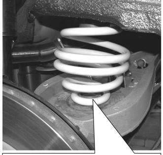
Install the factory upper spring perch between spring and transverse control arm.
