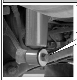
Use the supplied washer at the lower damper fixing point. Install the washer facing the center of the vehicle (as shown on the picture). The rear axle shock absorber hast to be installed according to the car manufacturers installation instruction.
