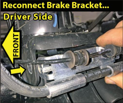
[Illustration 14] Reconnect factory brake line bracket from axle coil spring seat. [10mm]
