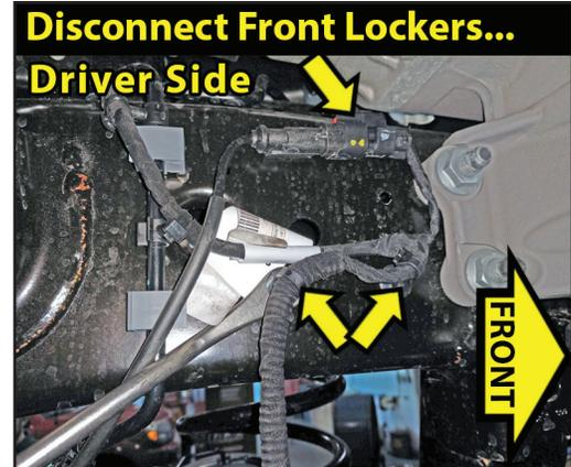
**UNCLIP CENTER AXLE DISCONNECT (CAD)...**
