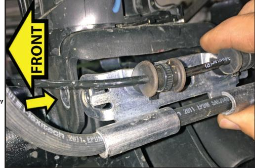
**Illustration 15****Install Front Shock Spacer...**
