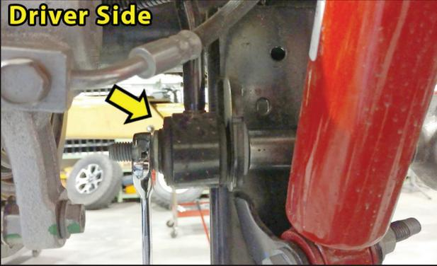
**Illustration 30****Disconnect Rear Shock at Axle...****Driver Side**
