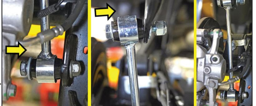
**Illustration 42****Install Links to the INSIDE of the Sway Bar...****Driver Side**
