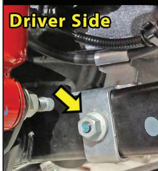
**Illustration 6****Disconnect Front Driveshaft...**
