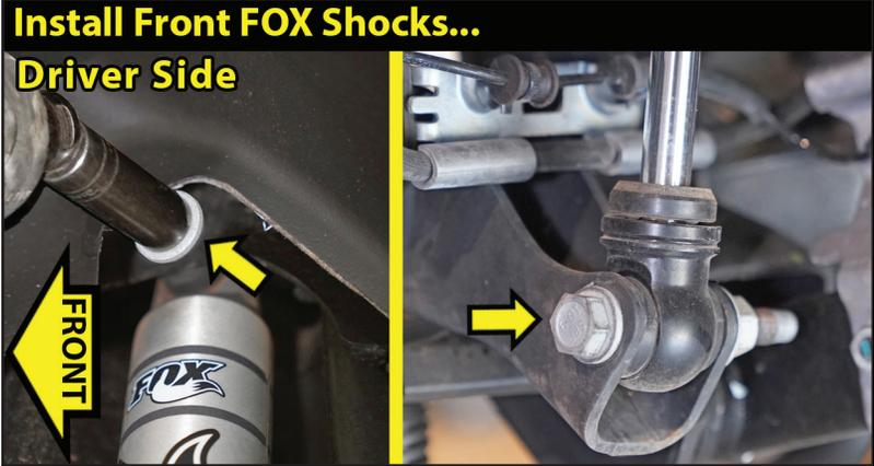
[Illustration 16] Locate the #985-24-177 FOX Shocks. Install the FOX front shocks using the factory hardware at the upper shock tower mount. Tighten the upper hardware until bushings swell slightly. [18mm socket]
