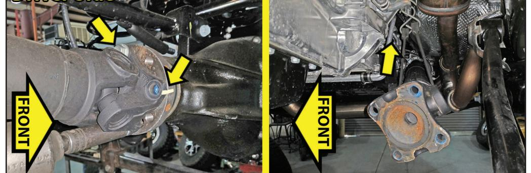
**DISCONNECT FRONT AXLE VENT TUBE...**
