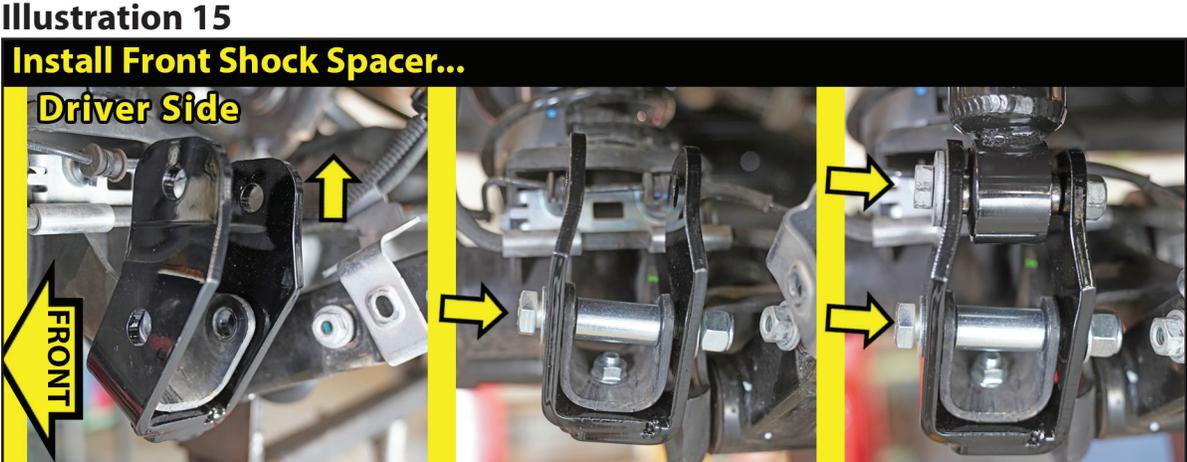
[Illustration 15] Locate the (2) SUPERLIFT front shock spacers (#55-13-5825). They are not side specific. Locate Hardware Bag #77-5800. Hardware PER Side: (1) #24-5704 Sleeve, 0.75" OD x 0.50" ID x 1.50" Long, (1) 3/8" x 1-1/4" Bolt, Coarse Thread, (1) 3/8" SAE Washer, (1) 3/8" Flange Nut, Coarse Thread (1) 1/2" x 3-1/2" Bolt, Coarse Thread, (1) 1/2" SAE Washer & (1) 1/2" Nyloc Nut, Coarse Thread.
