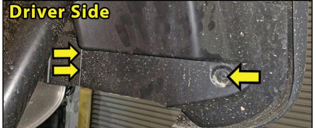
**Illustration 33****Disconnect Rear Shock at Frame...****Driver Side**
