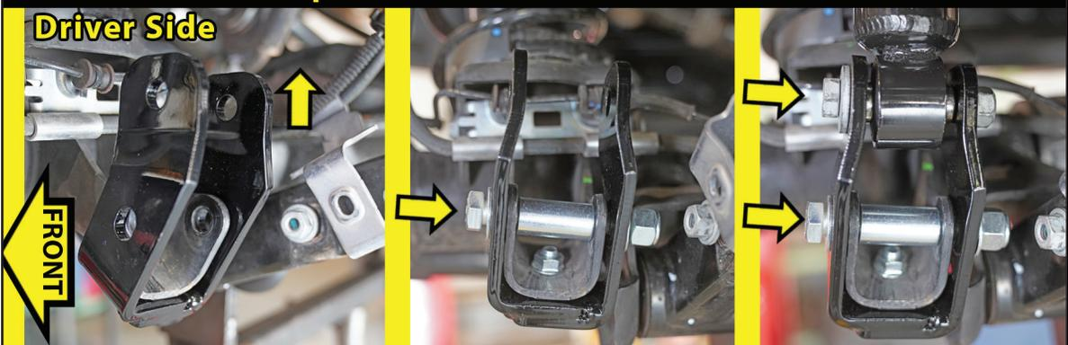
**TECH TIP** The bottom hole of the factory shock mount may have to be deburred before the bolt is installed easily. Use a 3/8" drill bit to deburr the hole if needed.
