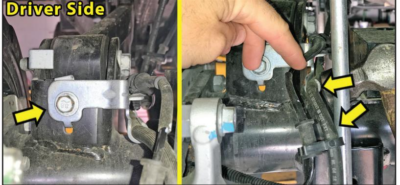
**Illustration 44****Reconnect Rear Locker...**
