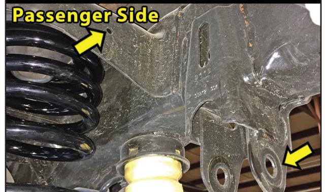
**DISCONNECT REAR SWAY BAR LINK AT AXLE...**
