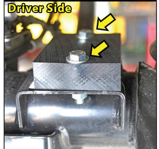
**Illustration 37****Install Rear Coil Spring with Isolator... Driver Side**
