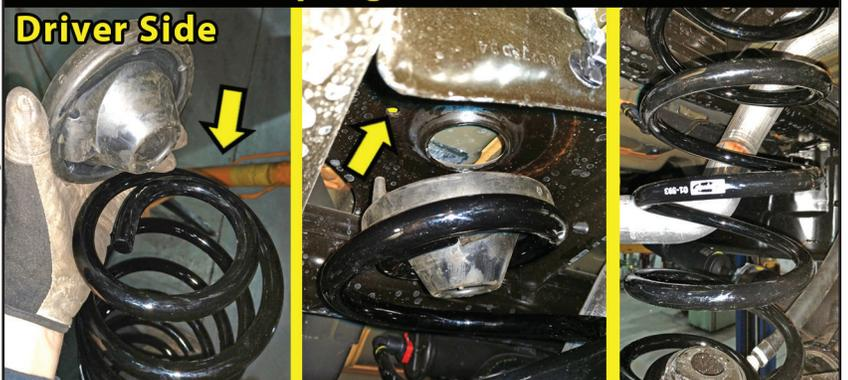
**INSTALL REAR SHOCK SPACER INSTALL...**
