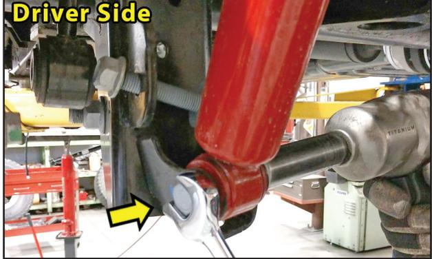
**DISCONNECT REAR SWAY BAR LINK AT SWAY BAR...**
