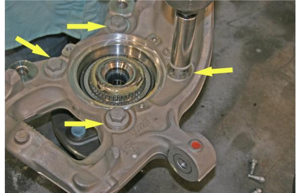
□□ [Illustration 52] Install the new knuckle (66-01-9930 driver's side and 66-02-9930 passenger's side) onto the hub bearing assembly. Apply thread locker to the factory hardware and install bolts; tighten. (151) {18mm}
