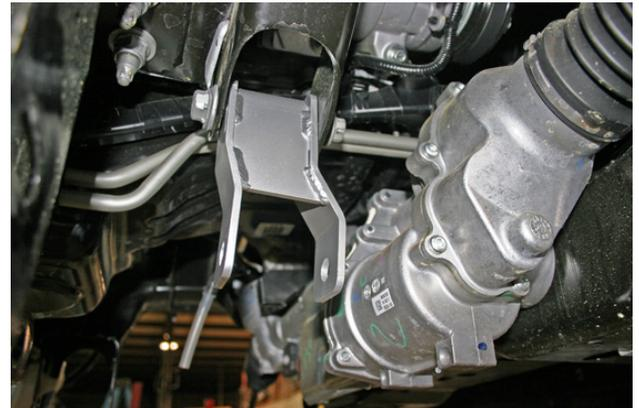
□□ [Illustrations 35 & 36] Position the front driver differential bracket into the frame using the factory hardware; install bolt from front, then pivot the differential into the passenger side differential bracket and secure using the supplied 9/16" x 3-3/4" bolts, washer, and nut; install bolt from rear. Do not tighten.
