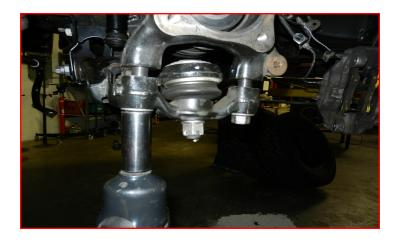
Remove the lower strut and sway bar hardware. Loosen but do not remove the lower control arm cams and let swing out of the way.
