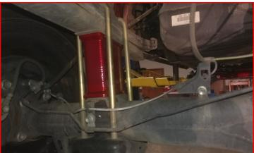
Remove the boot clamp from the shock and remove the boot from the shock.
