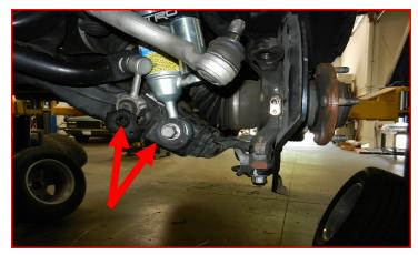
Remove the strut from the frame. Remove the ReadyLIFT strut extension. Make sure to mark them for reassembly later. These are driver and passenger side specific and must go back on their corresponding sides. Mark the spring location to shock body.
