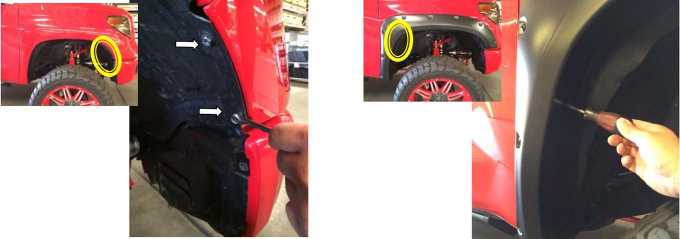
**STEP 7:** Using a 10mm socket / wrench, remove the 2 front screws from the inner splashguard front fascia area, retain these for later re-install.
