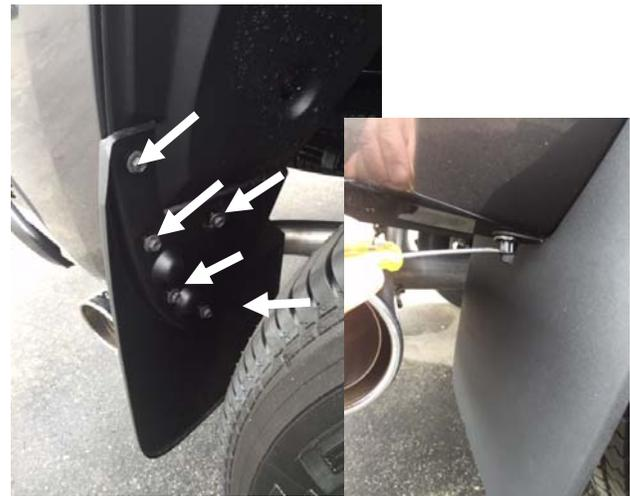
**STEP 13:** Using a 10mm socket / wrench remove the 5 screws from the inner area of the mud guard. Using a small flat screwdriver disengage the pin from the plug at the base of the mud guard. Remove mud guards completely and retain all components. Mud Guards cannot be installed with these Fender Flares.
