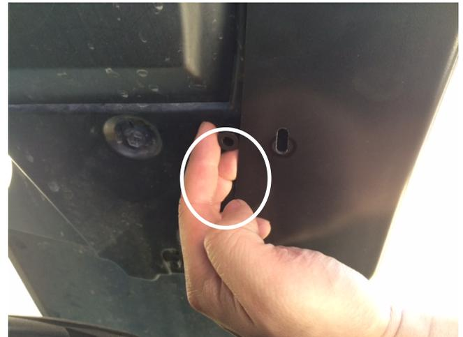
**STEP 17:** Note the (3) remaining open slot positions in the Fender Flare. Ready the spacers (and long screws) to go in behind the Fender Flare to fill the gap between the flare and the vehicle.
