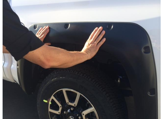
**STEP 14:** Clean the body area where the Fender Flares will make contact. Ensure fenders are dry prior to install.
