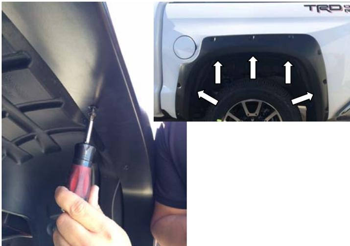
**STEP 16:** Loosely install a provided short screw into the top center hole in the Fender Flare. Continue installing the remaining (4) short screws into the 2 closest mounting locations either side of the top center hole. Do not fully tighten screws at this stage.
