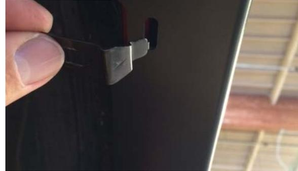
**STEP 10:** Locate the (3) remaining mounting slots on the Fender Flare as shown.
