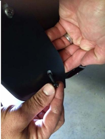
**STEP 18:** Working from top to bottom at these same (3) slot positions, hold and align the spacers with the slots and use the Long Screws to go through the spacers and into the corresponding factory holes. Do not fully tighten screws at this stage.
