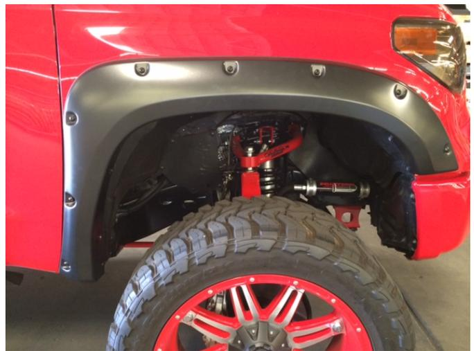
**STEP 6:** Hold Fender Flare on the vehicle in the position of best fit. Note where above marked slots in the Fender Flare, align with the existing screws / mounting holes in the vehicle. Make special note of "A" Remove the Fender Flare.
