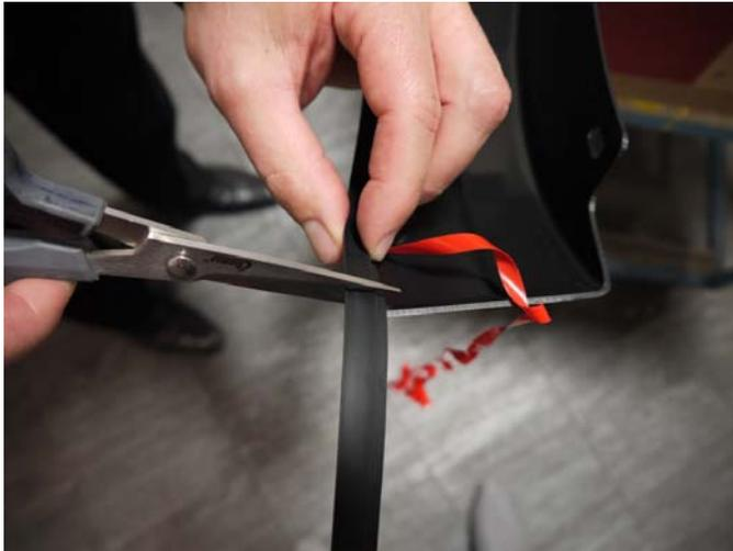
**STEP 3:** Trim rubber seal at end of each Fender Flare. Save extra rubber seal for install on opposite side Fender Flare and discard any excess once both sides are complete.
