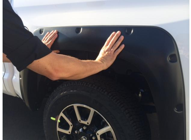
**STEP 19:** If necessary, make minor adjustments to the flare's position to achieve the best fit. Ensure rubber seal is sitting flat against vehicle. When satisfied, fully tighten all screw locations in the above order in which they were just installed. Repeat install for opposite side.
