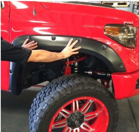
**STEP 12:** If necessary, make minor adjustments to the flare's position to achieve the best fit. Ensure rubber seal is sitting flat against vehicle. When satisfied fully tighten all screw locations, in the above order in which they were just installed. Repeat install for opposite side.
