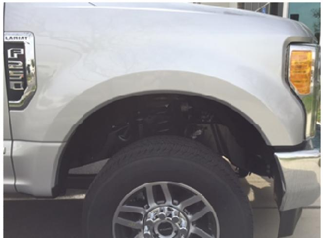
**STEP 4:** Clean the body areas where the Fender Flares will make contact. A light misting on fender using a soap and water solution can aid in proper rubber placement.
