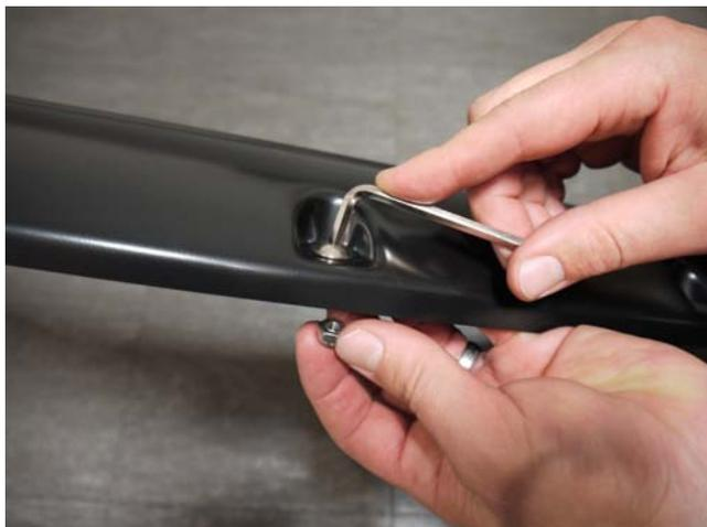
**STEP 8:** Attach bolts to each Fender Flare using a 3/16" Allen key and a 10.0mm wrench/socket. (wrench/socket and Allen key not supplied). Ensure inside of Fender Flares where the rubber seal is attached is clean, using the alcohol wipes provided. Wipe away any residue with a dry clean cloth.
