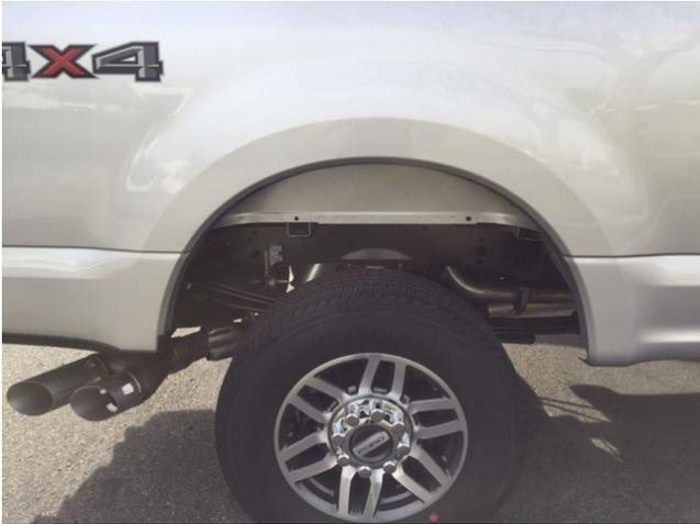
**STEP 10:** Clean the body areas where the Fender Flares will make contact. Use the supplied alcohol wipe. A light misting on fender using a soap and water solution can aid in proper rubber placement
