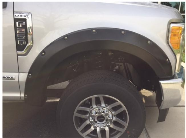
**STEP 6:** Place the Fender Flare onto the vehicle and fit into the correct position following the contours of the body. Ensure the slots in the part align with the holes in the fender from the previously removed 7/32 in socket head screws.
