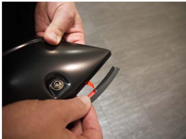
**STEP 9:** Attach the included rubber seal to the Fender Flares. Peel back 2" of the adhesive backing and position on the Fender Flare. Attach the seal to the Fender Flare, peeling back a few inches at a time. Attach rubber seal along all areas the Fender Flare will make contact with the vehicle body.
