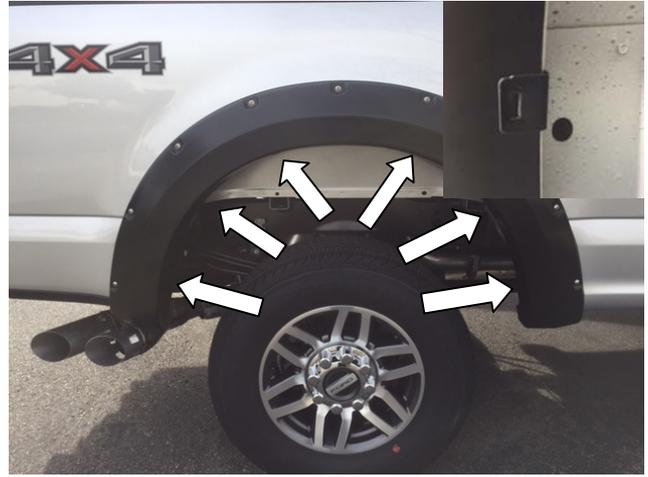
**STEP 11:** Place the Fender Flare onto the vehicle and fit into the correct position following the contours of the body. Use the twelve (12) provided "U" Shaped Retention Clips (six 6 per side) to secure the Fender Flare to the body. Make sure the dimple in the clip securely attaches in the slot on the Fender Flare.
