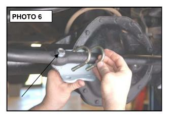
Locate and install the new center bracket as shown in **Photo 6** using the supplied  $\frac{1}{2}$ " bolt / hardware through the stock stabilizer mounting location and  $\frac{3}{8}$ " u-bolts on 02-07 models . **If the factory hole is not present in the tie rod the 1/2**" bolt will not be used. Make sure bracket is
