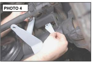
3. On drivers side secure with supplied ½" & 7/16" hardware .The supplied 7/16" bolt / flag nut is used as shown in **Photo 4**. Repeat for Passenger side as shown in **Photo 5** and secure with supplied 7/16" hardware for the stock mounting location and ½" for the lower drilled hole.
