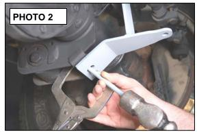
2. Locate the new driver side stabilizer bracket. Align top hole and hold in place with clamp as shown in **Photo 1**. Mark as shown with ½" transfer punch and drill hole using a ½" drill bit as shown in **Photo 2 & 3**. Repeat on passenger side.
