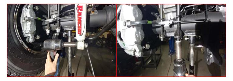
Remove the rear shocks. Support the axle with a suitable jack. Loosen but do not remove the driver side u-bolts. Remove the passenger side u-bolts completely and lower the axle.
