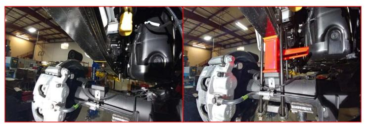
Install the ReadyLIFT passenger side block (if tapered, make sure the taper goes towards the front of the vehicle) (make sure the offset pins locate the axle to the front of the vehicle) and raise the axle lining the center pins up. Install using the provided u-bolts but do not fully tighten at this time. Repeat steps for the drivers side.
