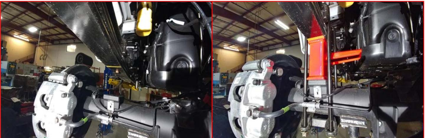
Install the ReadyLIFT passenger side block (if tapered, make sure the taper goes towards the front of the vehicle) (make sure the offset pins locate the axle to the front of the vehicle) and raise the axle lining the center pins up. Install using the **provided u-bolts** but do not fully tighten at this time. Repeat steps for the drivers side.
