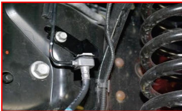
**2017 - UP front brake line:** Install the ReadyLIFT brake line bracket to the factory brake line using **5/16" x 3/4" bolts, washers, and nuts**. Install the bolt facing outwards. Torque to **10 ft-lbs**. Gently pull the metal brake line down while lining up the ReadyLIFT bracket to the original holes in the frame. Install using **factory hardware**. Torque to **5 ft-lbs**.
