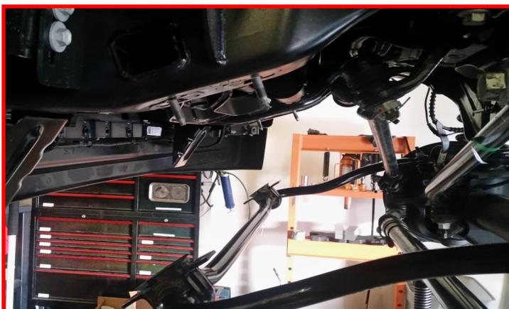
Loosen but do not remove the radius arm bolt at the frame. Lower the axle enough to remove the front springs. Make sure not to over extend the ABS, brake lines, and vent tube. Install the ReadyLIFT urethane isolator, spring spacer, and then factory rubber isolator onto the spring. Raise the axle enough to hold the spring assembly in place.
