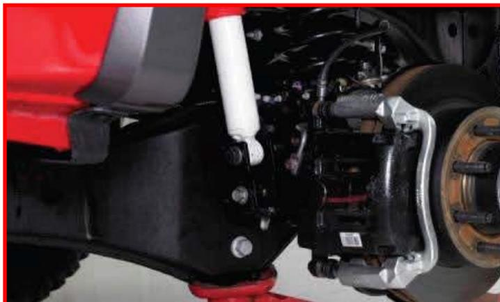
Install the ReadyLIFT shock extensions to the axle using factory hardware making sure the offset hole is towards the rear of the axle. Install the shock to the ReadyLIFT shock extensions using the **M14 x 70mm bolt, washers and nuts**. Torque to **45 ft-lbs**. (2017 and up models shown, earlier models differ slightly. The offset hole will end up towards the radius arm.)
