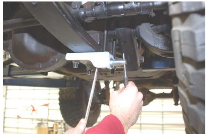
17. Install new brake lines in stock hole locations reusing the T45 torx head bolt on frame rail for the new supplied bracket.
