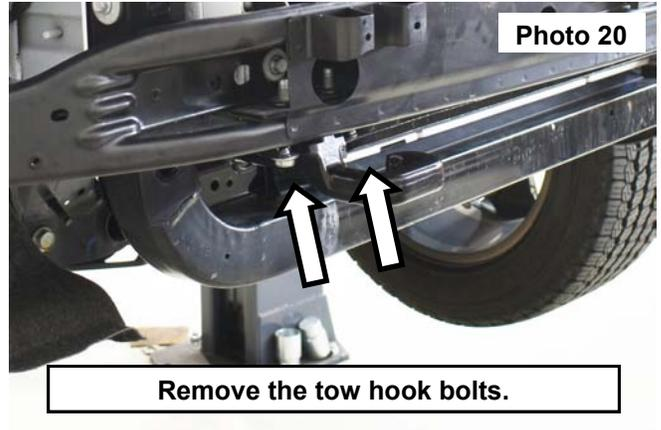
20. Remove the tow hook from the vehicle, set aside for reuse. **See Photo 21.**
