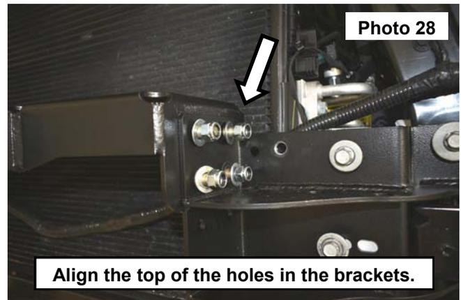
27. Torque the 4 bolts installed into the winch plate and the brackets to 45 ft-lbs, use a 5/8 wrench and socket. **See Photo 29.**
