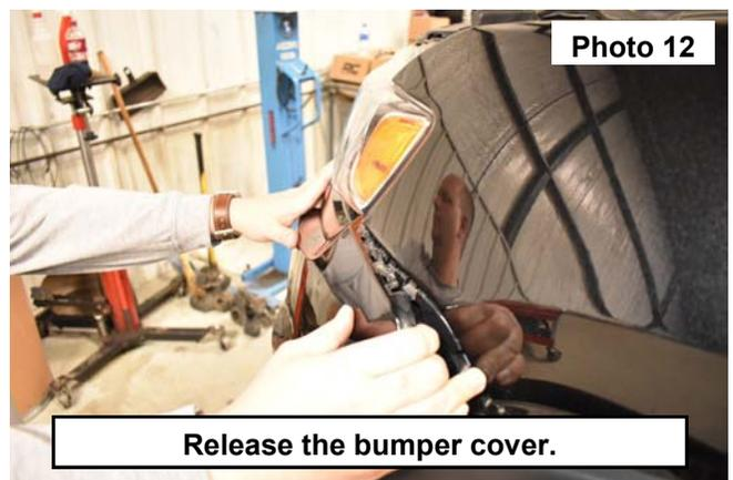
12. Remove the bumper cover from the vehicle, set aside in a safe place for later modification. **See Photo 13.**
