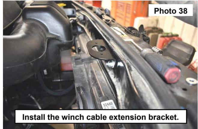
38. Install the winch cable extension into the bracket installed onto the radiator support, using the supplied #8-32 x 1 socket head bolt, #8 flat washer and a #8-32 nut. **See Photo 43.** Tighten using a 9/64 allen wrench and a 8mm wrench.
