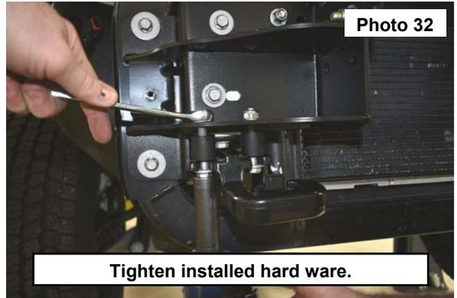
32. Install the nut on the back side of the tow hook, tighten using a 30mm socket. **See Photo 33.**
