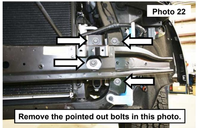
22. Remove the 2 bolts on each side of the crash bar, use a 13mm socket. **See Photo 23.** Retain hardware for later use.
