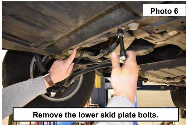
6. Remove side the bolts, on each side of the skid plate, using a 10mm socket. **See Photo 7.** Save hardware.
