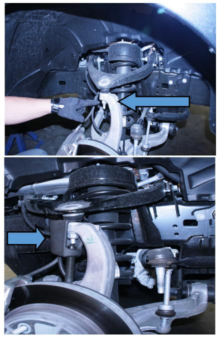
8. Remove the lower strut bolt and nut. Retain the factory lower bolt for reassembly. Note the direction of the bolt for reassembly
