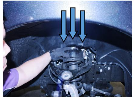
10. Remove the strut from the upper strut tower so you can install the spacer.
