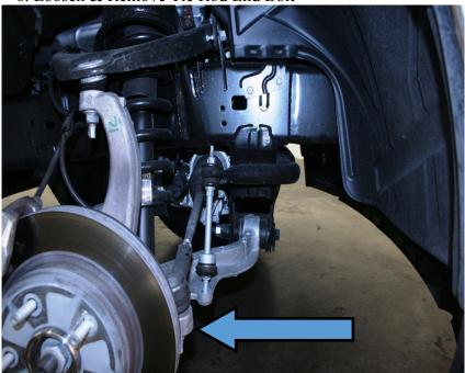
7. Remove the upper ball joint nut and separate the knuckle from the upper A-arm using the appropriate Puller tool
