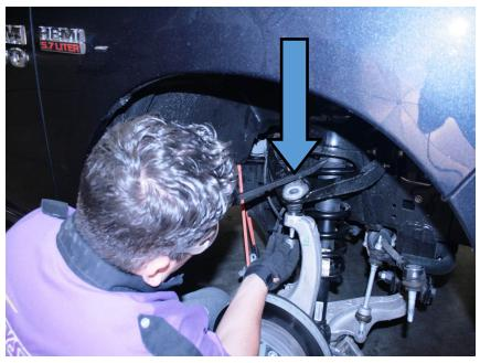
17. Reconnect the lower tie rod end first, & Then the sway bar
