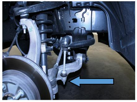
6. Loosen & Remove Tie Rod End Bolt
