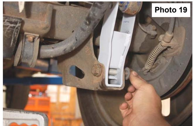
The stock shocks will be installed after the vehicle is lowered to the ground using stock hardware.
