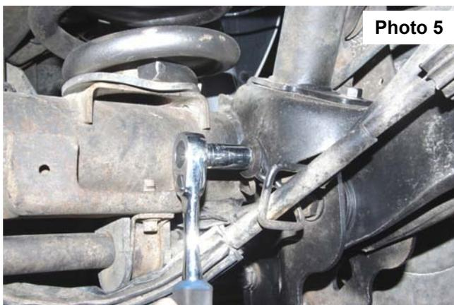
12. Install the supplied control arm drop bracket into the factory control arm pockets on the frame. Use the factory hardware in the lower mount to hold the bracket. **Do Not Tighten. See Photo 6.**
