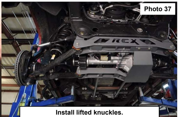
45. Install the wheels and tires, then jack up the truck and remove the jack stands. Lower truck on ground tighten upper and lower control arm bolts using 21mm for upper and 18mm and 24mm socket and wrench for bottom. **Torque to factory specs.**
