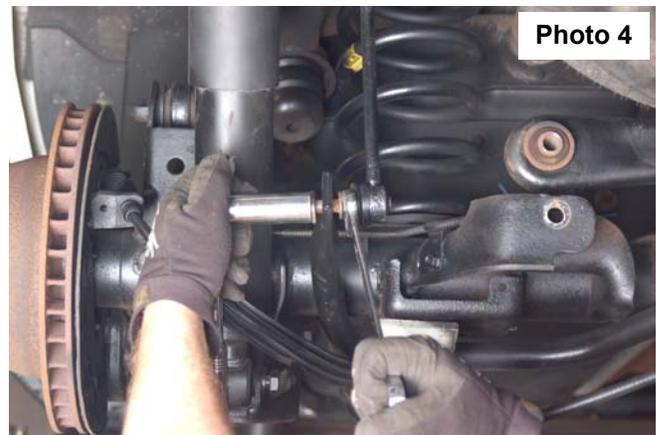
8. Remove the lower shock from the axle using a 21mm wrench/socket leaving the upper part of the shock attached to the frame. Retain the hardware for reuse.
