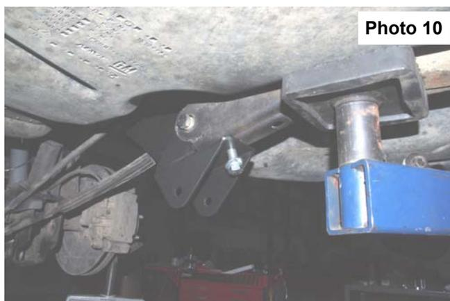
17. Install the upper control arm in the control arm drop bracket using the supplied 9/16" x 4" bolt, washers, and nut (1287BAG1) and on the axle using the factory hardware. **Do Not Tighten. See Photo 11.**
