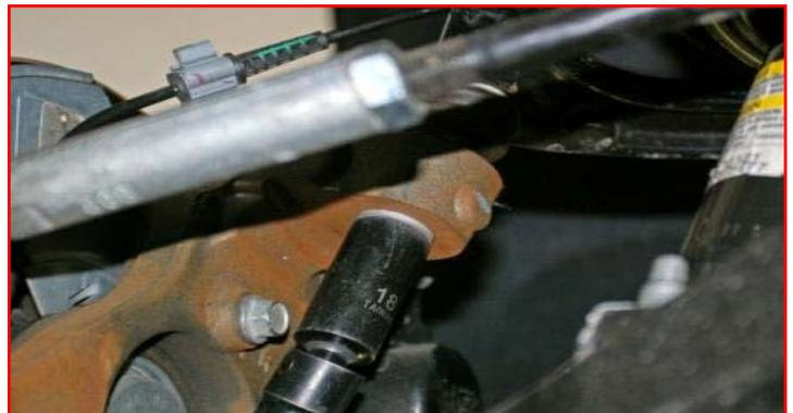
**4wd only:** Install the CV axle to the hub bearing using the **factory hardware**. Torque to **200 ft-lbs**. Re-install axle nut cover by tapping into place with a mallet on the outer edge.
