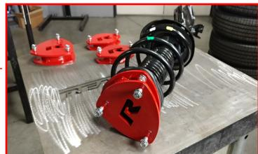
When installed correctly, the R logo will be legible through the strut tower when facing the engine compartment from the side that you are on. Passenger side shown. The spacers are offset to the inside and rear of the vehicle to adjust for camber and caster.
