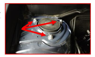
Locate the ReadyLIFT front strut extension. These are driver and passenger side specific. Passenger side shown. Install to the top of the strut using the factory hardware. Torque to 30 ft-lbs.
