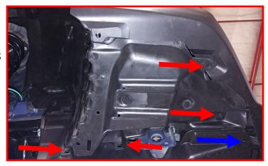
Pull the skid plate down to access the bolt holding the last of the inner fender liner. Remove and discard. Reinstall the plastic push clip into the skid plate.
