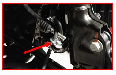
Install the ReadyLIFT sway bar bracket to the strut using the provided M12 bolts, washers, and nuts. Install the factory end link to the ReadyLIFT bracket using the factory hardware. Torque all to 45 ft-lbs. If you have not started the opposite side of the vehicle at this time, you may not be able to line the sway bar up until the opposite side is released.
