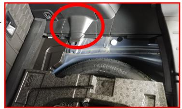
Remove the strut nuts and set aside.
