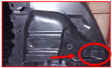
Once this is achieved, you can push the liner forward. Line up the back edge of the liner with the bumper cover. Drill a new hole into the liner. Install a plastic push clip.
