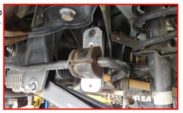
Install the sway bar to the brackets using the factory hardware and factory pinch bracket. Make sure to install the factory pinch bracket with the locking tang down. Torque to 25 ft-lbs.
