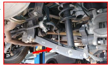
Remove the sway bar at the subframe and let hang out of the way.
