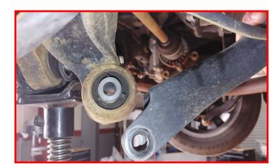
Loosen but do not remove the lower control arm bolt at the subframe. Remove the lower strut bolt on the lower control arm and the control arm bolt at the knuckle.
