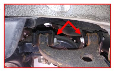
Loosen but do not remove the front lower control arm bolt at the subframe.
