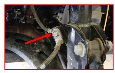
Install the ReadyLIFT sway bar bracket to the strut using the provided M12 bolts, washers, and nuts. Install the factory end link to the ReadyLIFT bracket using the factory hardware. Torque all to 45 ft-lbs.
