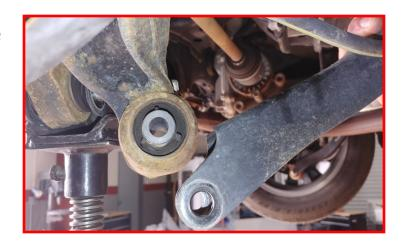
Install the ReadyLIFT sway bar brackets to the subframe using the provided M8 counter sunk bolts and a drop of thread locker. Torque to 25 ft-lbs.
