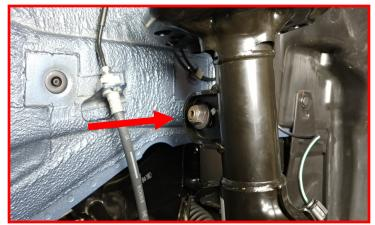
Remove the brake line bracket at the strut body. Let hang out of the way.
