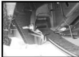
Support the frame with jack stands. The axle should also be supported with jack stands. A jack in the center of the axle will be used to raise or lower the axle when needed.
