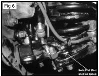
Install two  $\frac{1}{2}x20x3\frac{1}{2}$  bolts up through the bottom of the control arm and attach nuts on top. Hand tighten.
