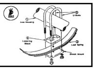
Install 3" block with pinion shim on top, with the thick end to the rear.
