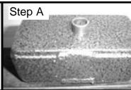
**B:** Place the ring shim on top of the leaf spring. Place block flat on spring. Lower axle down on the block. Be sure pin is aligned. Install u-bolts and tighten. Dakota RT require the holes in the factory spring plates must be enlarged to 5/8". Trim excess ubolt as needed.
