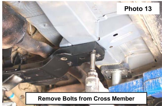
24. Lower cross member carefully leaving bolts installed but loose on one side. Install the transmission cross member spacers as shown in **Photo 14** and secure with the supplied 10mm x 140mm (approx. 5.5") bolts and washers from Bag 4 and re-using the stock outside factory bolts on the inside mount.
