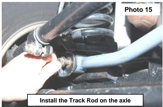
26. Assemble the spacers on the heim joint and install the track bar with supplied 12mm x 65mm (approx 2.6") bolt & flange locknut from track rod kit bag. Tighten using a 18mm & 19mm socket / wrench. **See Photo 16.**
