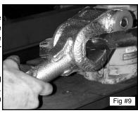
Install new shocks with  $1\2$ " x 2-3\4" bolts supplied. Review installation and check that all bolts are tight and installed correctly. Now you can tighten torsion adjustment bolt to the marks made earlier.
