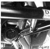
Cleaning the end of the torsion bar and removing the powder coating will make the torsion bar fit much easier into the new arms.
