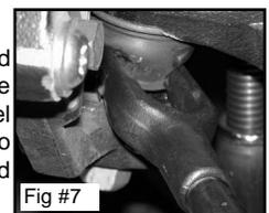
Using the floor jack, slowly lower the control arm until the tension is removed from the torsion bar.
