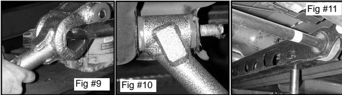
Raise the control arm to ride height (flat with the ground). Slide torsion key up into cross member and move torsion bar back to align with key. Install torsion adjustment bolt, do not tighten yet(Fig #11).
