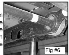
Place a floor jack under lower control arm and raise slightly. Remove lower ball joint nut. Free the lower ball joint from the spindle (Fig #7). All wheel drive and 4wd will require removing front axle so not to damage CV boots. Remove tie rod end from spindle.
