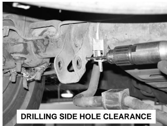
**DRILLING SIDE HOLE CLEARANCE**
