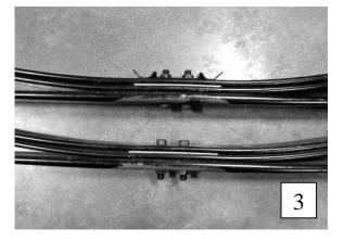
to hold the spring pack together while you reverse the center bolts, or loosen them and reverse one at a time. (**Photo 4**). Tighten the center bolts using pliers to hold the round head of the bolt.
