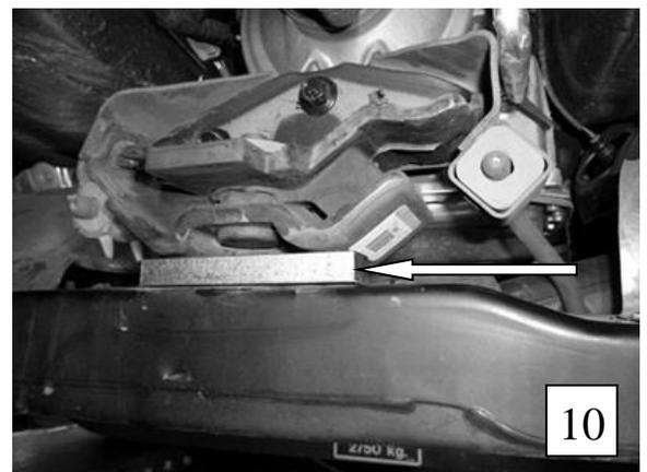
**For models with two piece driveshafts** you will need to re-locate the center carrier bearing mount.
