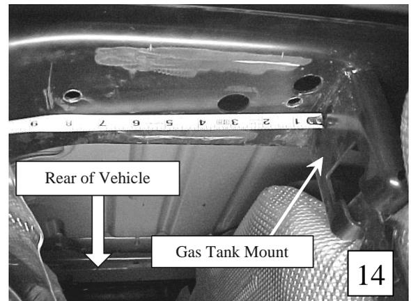
be drilled thru the lower portion of the cross member because of the cutout directly above it. The second hole furthest away from the gas tank mount will need to pass thru the lower and upper section of the cross member (**Photo 14**).
