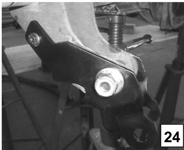
6b) Install Belltech Street Performance or Nitro Drop 2 shock to each side and torque to OEM specifications. See the current Belltech Application Guide or contact you nearest Belltech dealer for the appropriate part numbers for your application.
