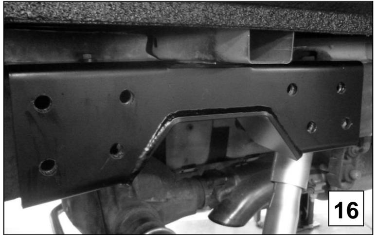
**4j)** With the C-section installed tightly against the outside face of frame rail, use the drill and a 1/2" drill bit, to transfer the (7) (drivers side), or (8) (passenger side)) 1/2" holes to the frame rail. Use the C-section holes to locate the drill bit. Repeat the drilling process on the inside of the frame.
