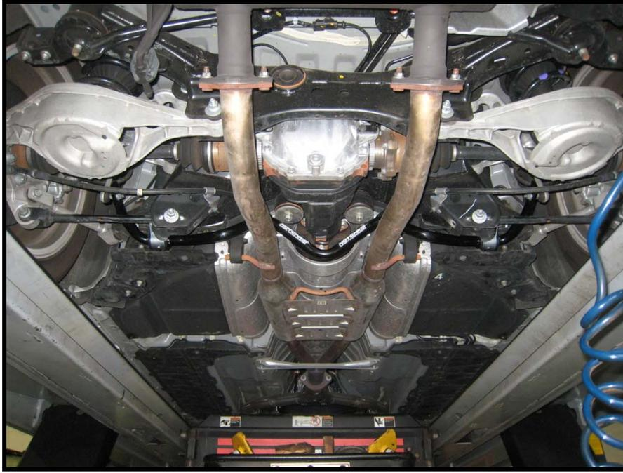
**IMPORTANT:** For maintenance, use the zerk fittings to grease the bushings at least once a year (15,000 miles) or when excessive noise occurs. Use a silicone based grease only! A lithium-based grease can wash out with water and should not be used.
