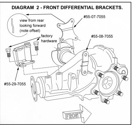
Use stock hardware to loosely attach the 3 Superlift differential brackets to the differential; the furnished 7/16" hardware secures the brackets' upper ends. All differential bolts are tightened later.
