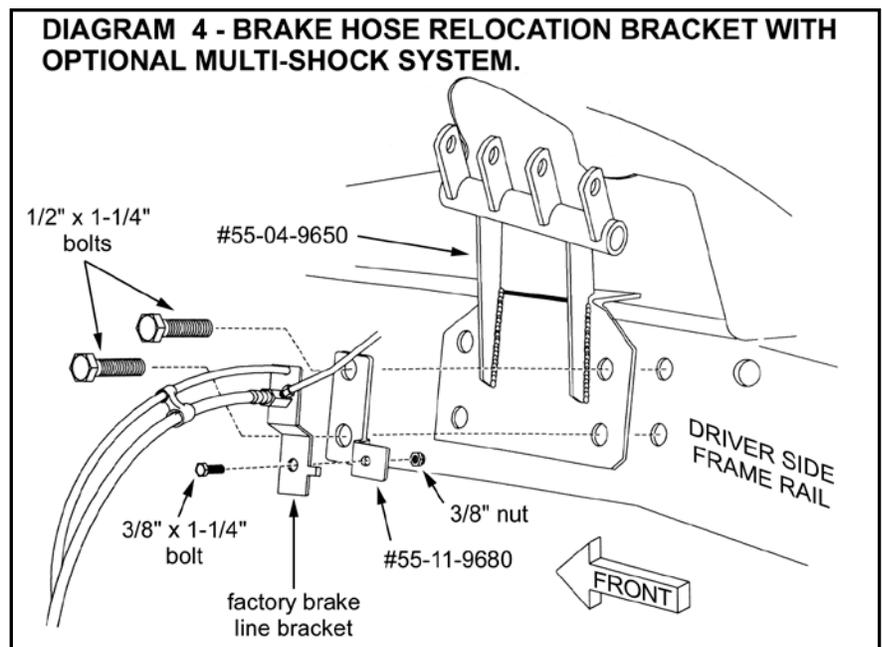
line. Remove the bolt securing this bracket to the frame.
