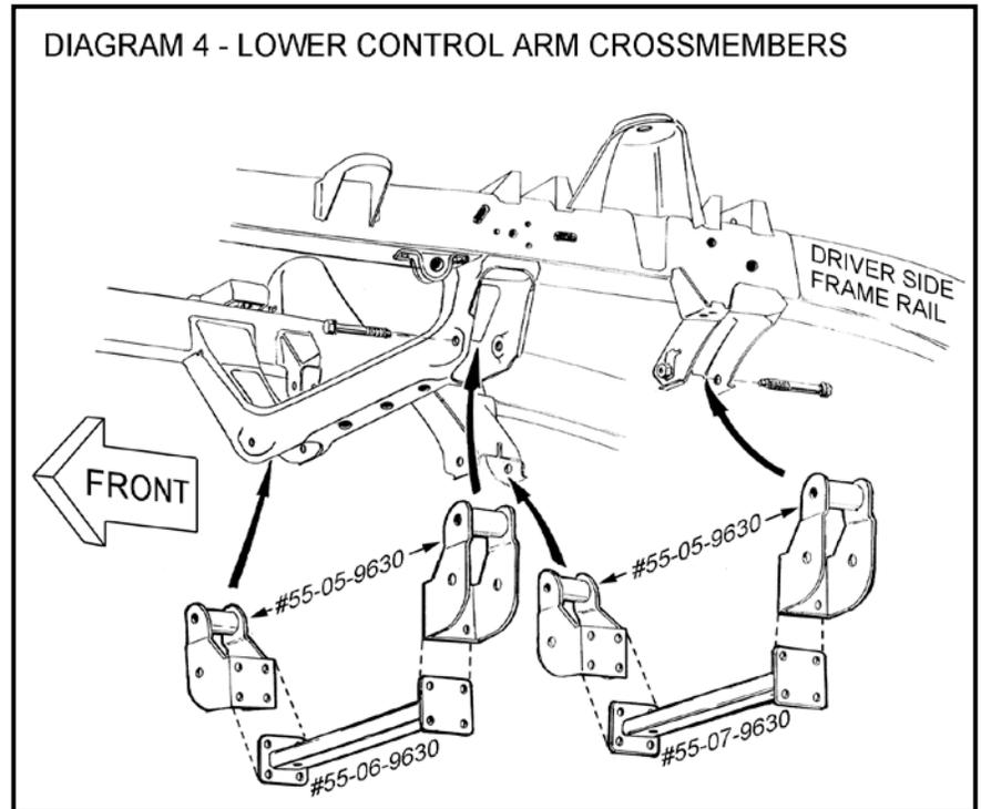
Except where noted, Steps 13 through 19 are performed one side at a time. Start at the driver's side.
