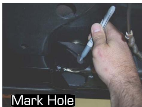
Weld-In: Mark the front subframe to indicate where you should grind/sand the paint for welding. The connector hole will allow you to apply a rosette weld instead of a bolt. You may also want to mark where the leading edge of the connector lies on the subframe so you can run a weld bead there as well.
