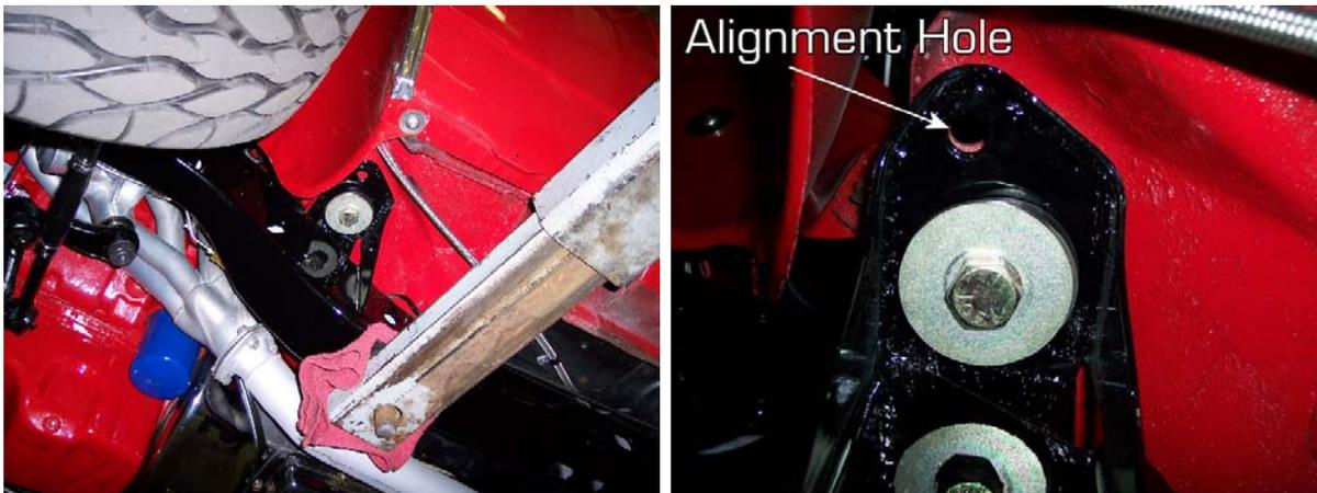
3 – The subframe connectors must be installed on an alignment rack or floor ramps (all 4 wheels). The vehicle must be sitting on it's wheels at ride height in order to install the subframe connectors. Do not use a two-post lift, as this will load the chassis/body in the wrong points causing the chassis to tweak.
