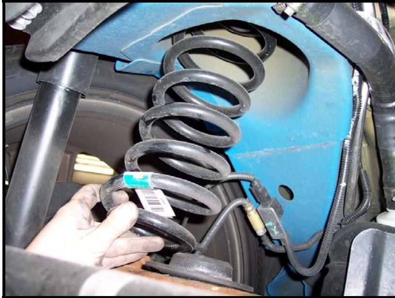
5. Install the new Hotchkis coil spring.
