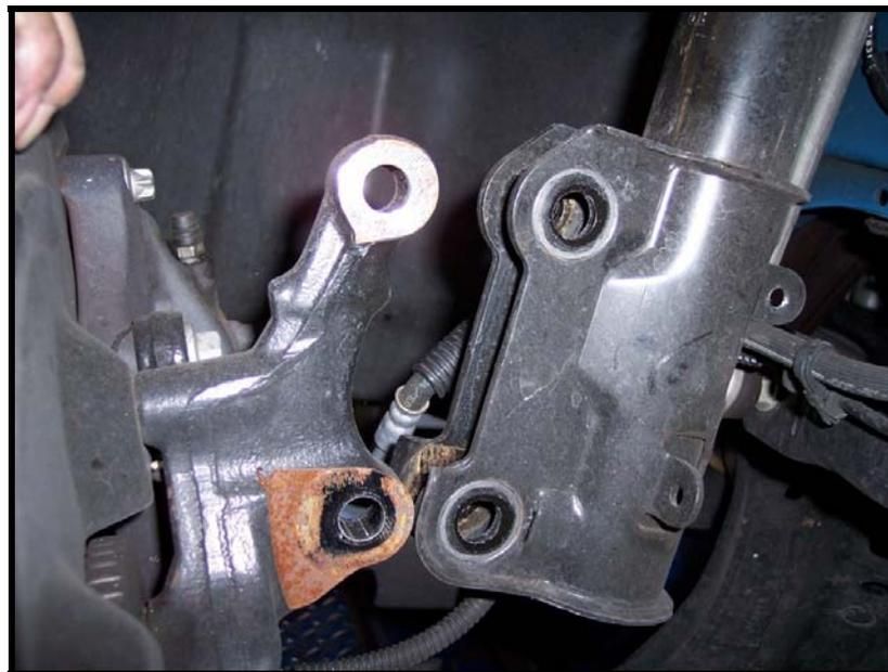
6. Either use wire or something else to restrain the spindle so the brake line and ABS sensor wiring does not get pulled on.
