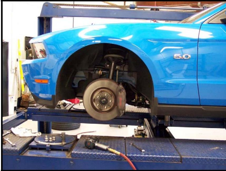
2. Remove the brake line bracket.
