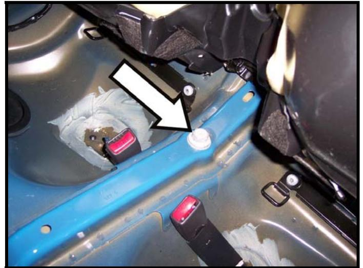
10. Connect the lower mount to the differential. To make the bolt align properly during installation, you may need to lift up the differential as shown below.
