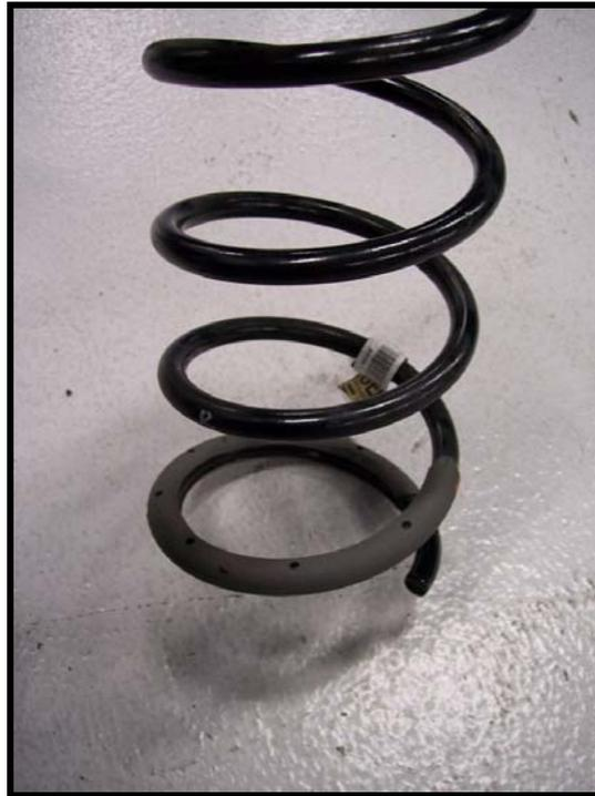
11. Remove the coil spring isolator from the old stock coil spring and install it on the new Hotchkis coil spring at the same position.
