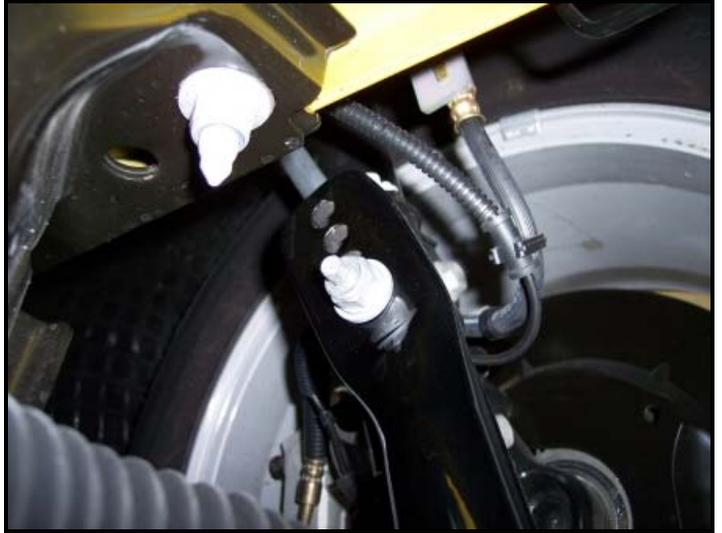
**7F Install Hotchkis Bushing onto the sway bar**
