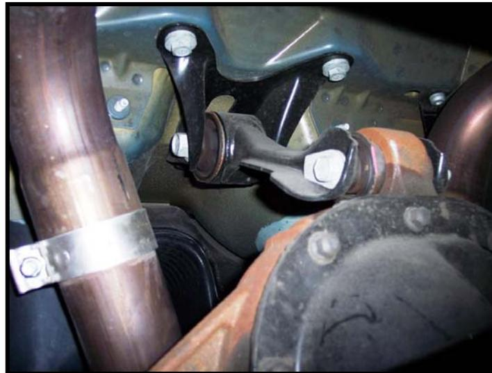
6. Remove the remaining two (2) bolts for the upper mount to the upper trailing arm.
