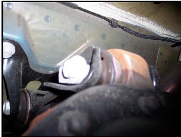
8. Remove upper trailing arm from upper mount and adjust the Hotchkis adjustable upper trailing arm to the same center to center length as the stock upper trailing arm. Tighten the jam nuts. Fine adjustments can be made later to set the pinion angle. Details of this is at the end of the installation instructions.
