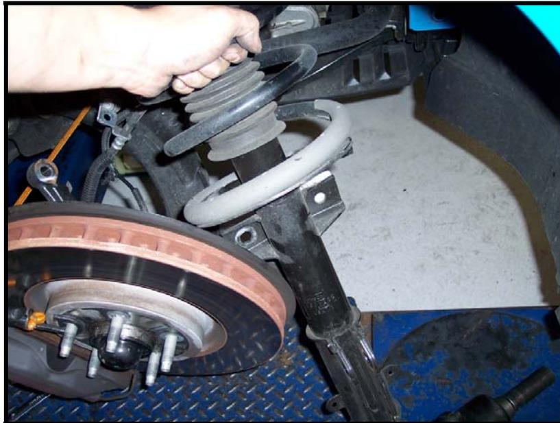
9. Using a spring compressor, compress the spring and remove the upper spring cup nut.
