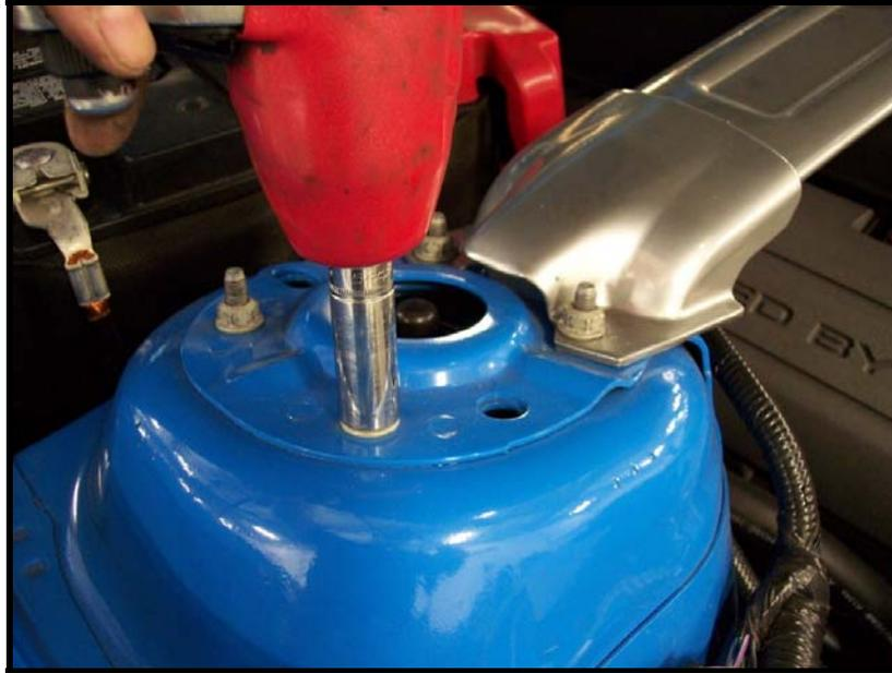
8. Safely remove the strut assembly.
