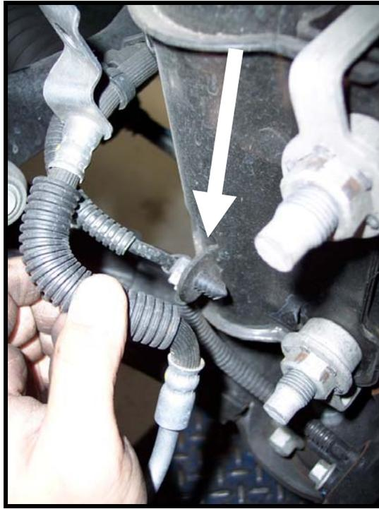
4. Unbolt the sway bar link and remove.
