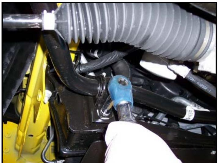
**4F Remove Endlinks and Remove Bar**
