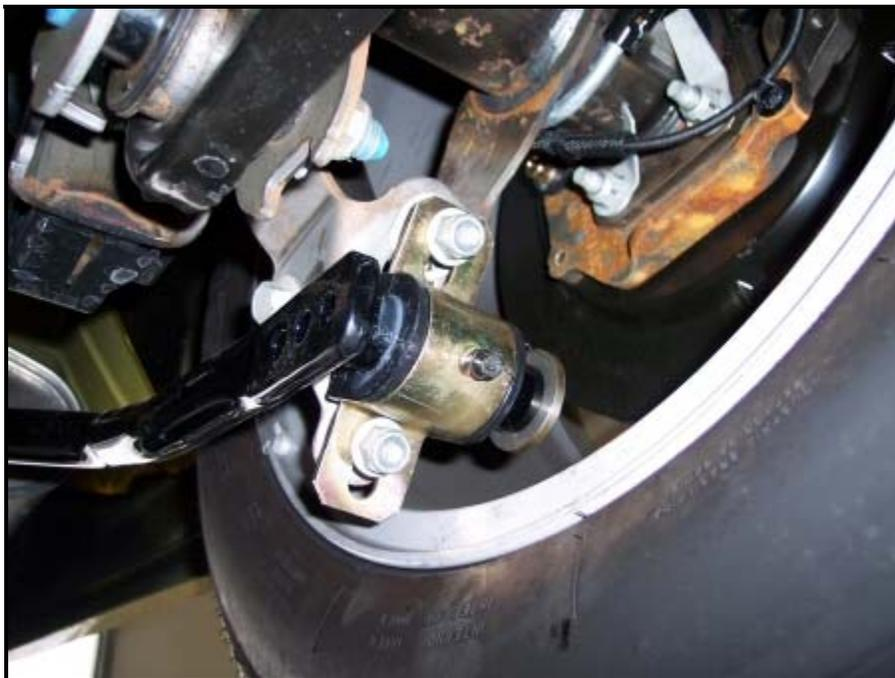
**11R Attaching Sway Bar to Axle Mounts**
