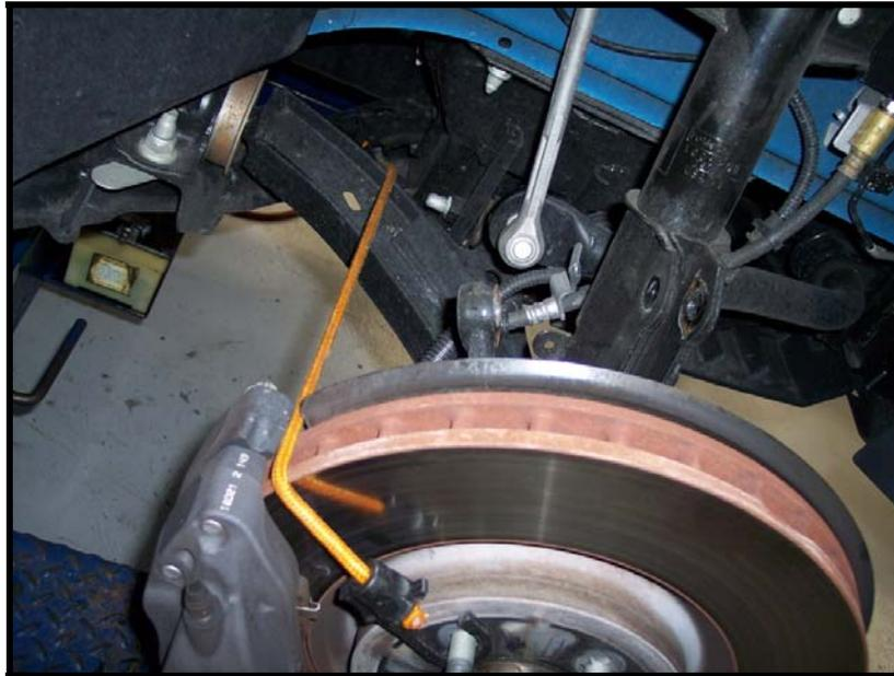
7. Now remove the four (4) upper mounting nuts for the strut. Just before removing the last nut, support the strut to ensure it from not falling.
