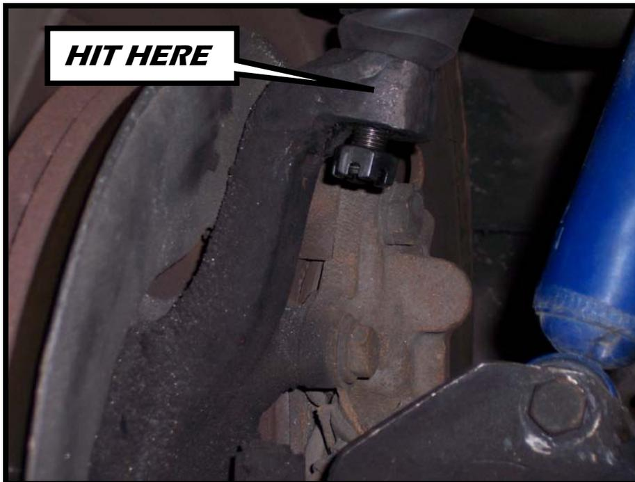
4. Support the suspension with a floor jack to relieve the pressure from the castle nut. Remove the castle nut.
