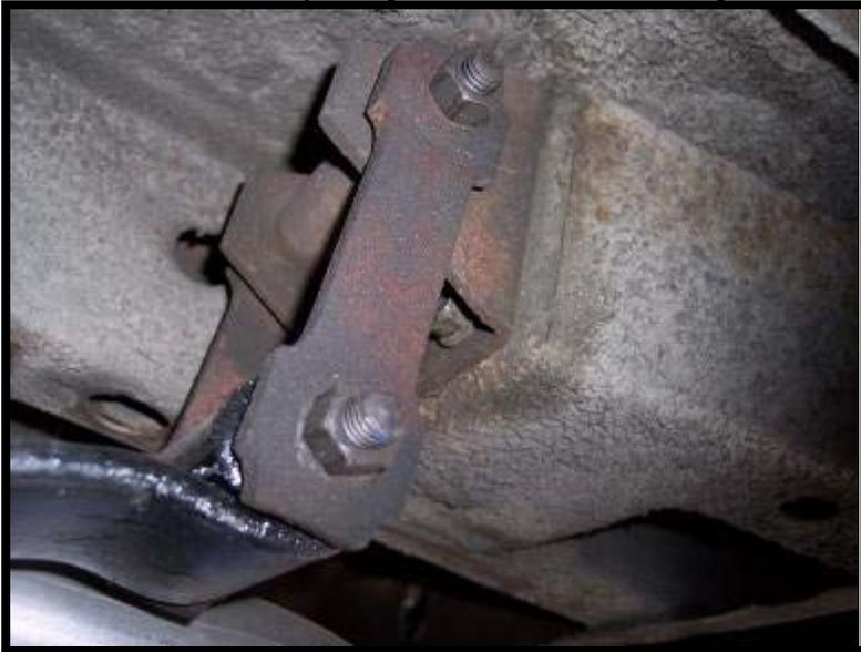
6. Support the spring with a stand and remove the 4 nuts on the front bracket.
