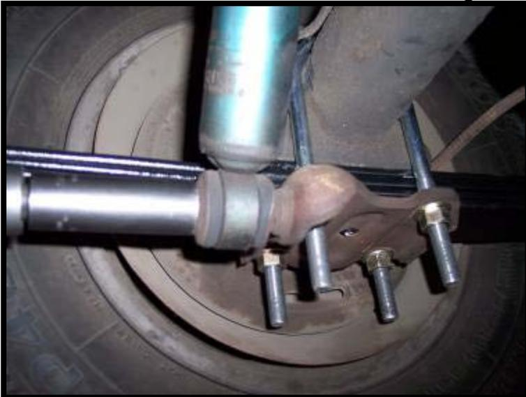
4. Now remove the lower shock mount plate from the U-bolts.
