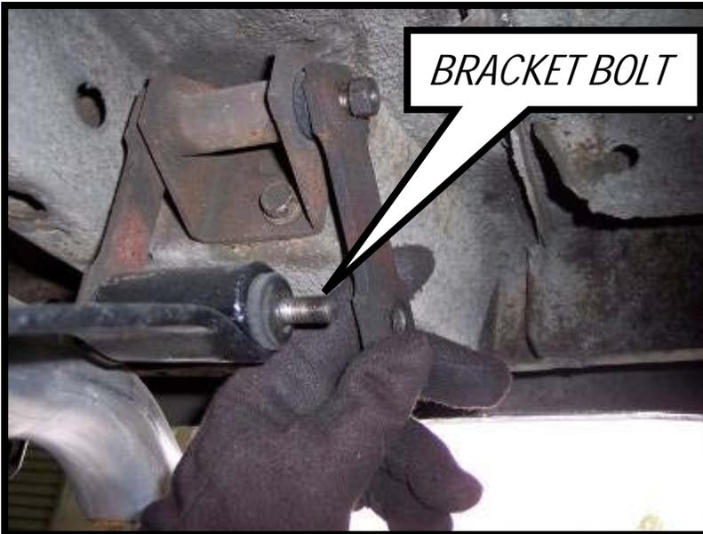
8. Install the new Hotchkis front bracket and bushings.
