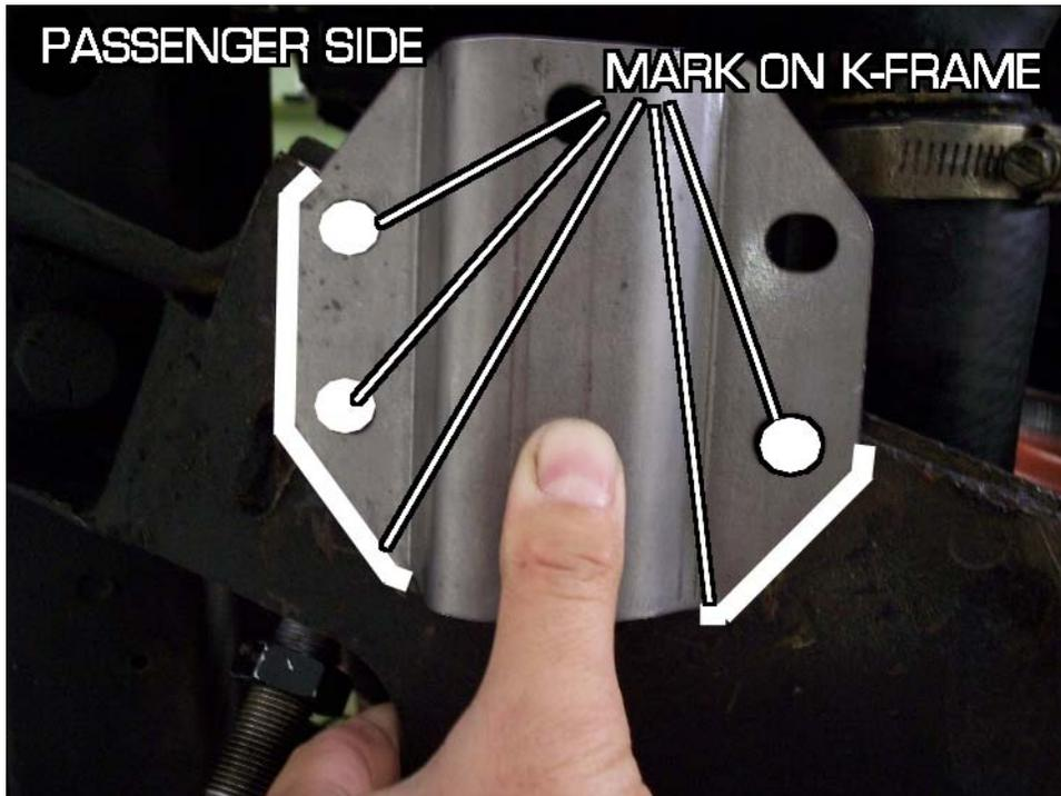
Once the k-frame is marked, use an angle grinder with a sand paper attachment to remove all of the paint and grime on the areas previously marked. What we are doing is cleaning the area that is going to be welded.
