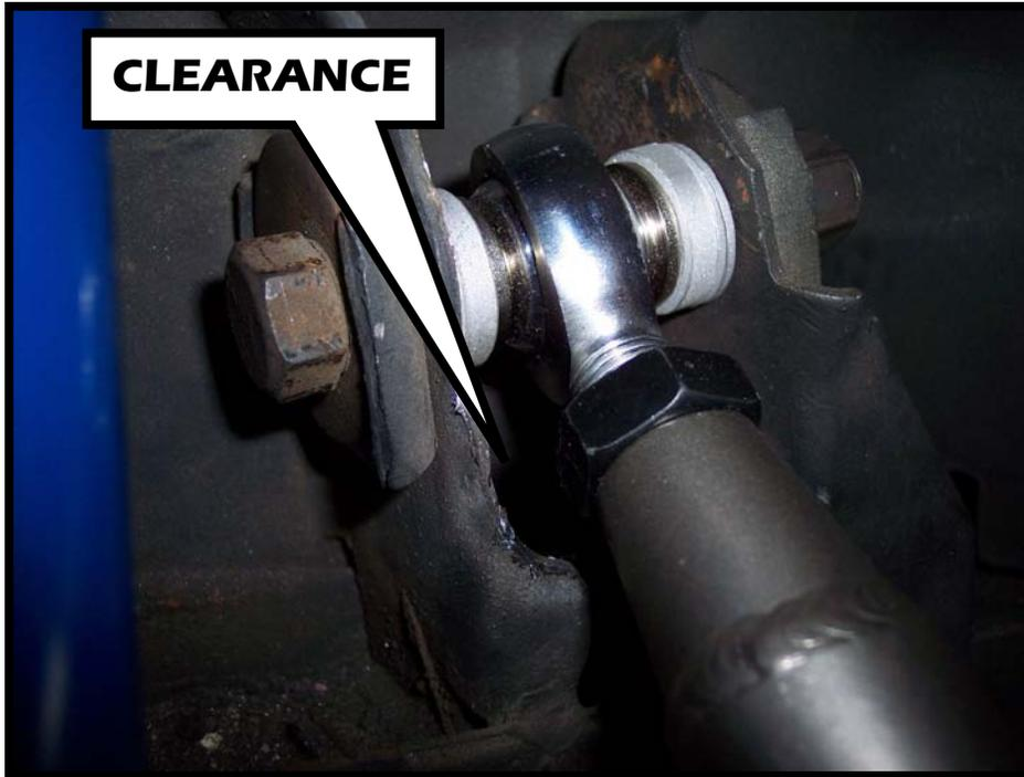
9. **Install the new A-Arms by following the same instructions in reverse order. When bolting on the rod ends, be sure to use the provided spacers.**
