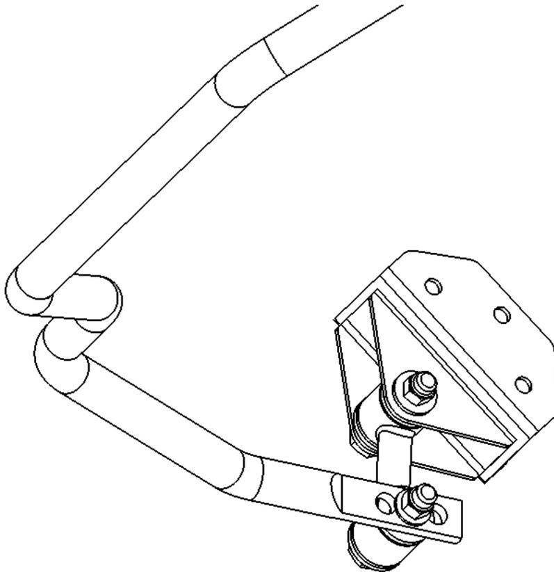
4R Rotate sway bar, and frame brackets up until they contact the frame rails. (Fuel lines, and parking brake cables may need to be loosened, and moved for proper placement of frame brackets, and can be re-installed when finished.)
