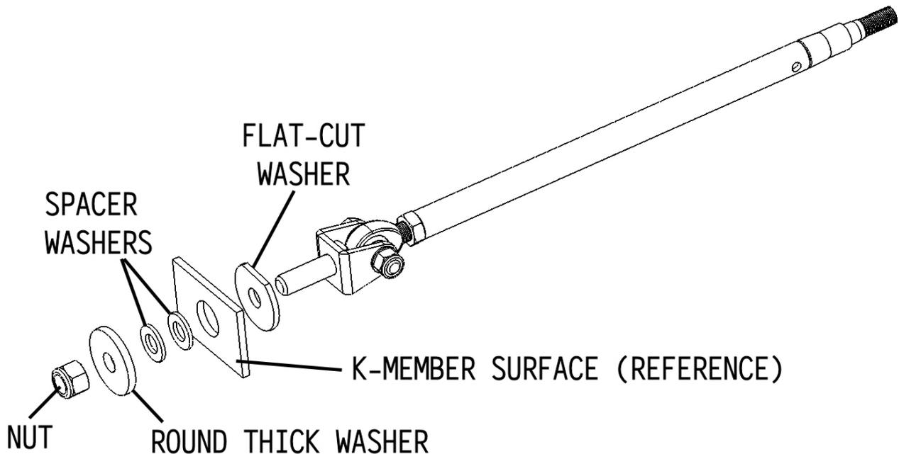
Install the large flat-cut washer onto the clevis stud and insert the front mount into the k-member hole.
