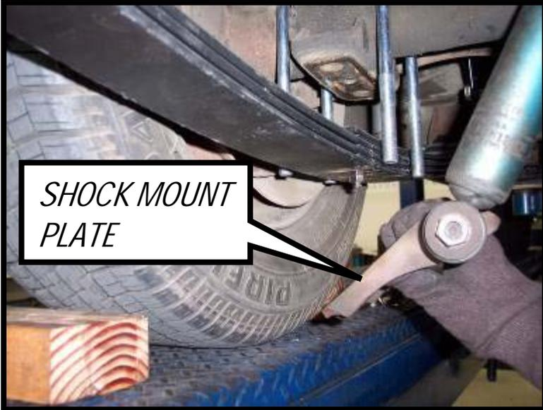
5. Loosen the two rear bracket nuts.
