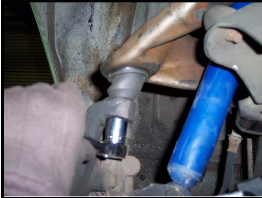
3. With the castle nut loose, hit the upright mount with a hammer until the spindle & the rest of the suspension pop loose from the A-Arm ball joint.
