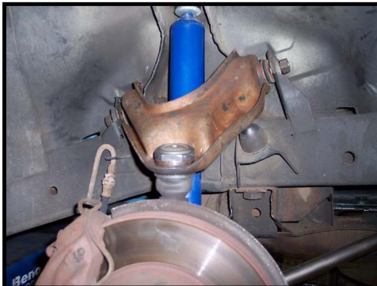
2. Remove the cotter pin from the ball joint and loosen the castle nut.
