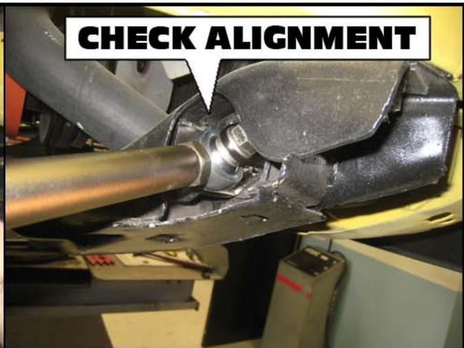
Restore torsion bar snap ring. Adjust the torsion bar tensioner back to where it was for proper pre-load.
