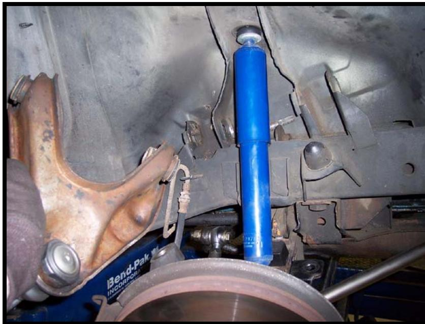
7. Adjust the rod ends on the Hotchkis A-Arms so they are set to .33 inches as shown.
