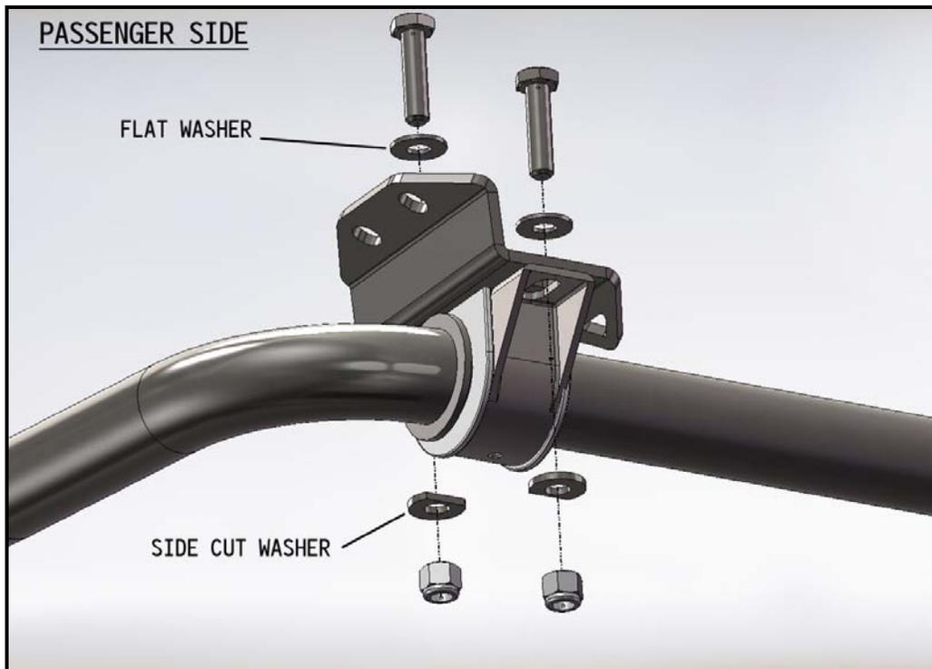
Position the entire assembly up to the K-member. The bracket should mate up to the k-member as shown below.
