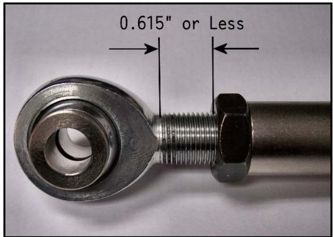
Center the heim joint so that it is not twisted one way or another. Tighten the heim joint jam nut.
