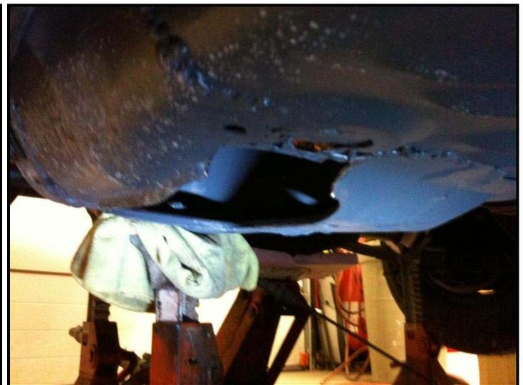
In addition, you will notice it will be extremely difficult to access the leaf spring mount nuts once the subframe connector is in place. To alleviate this problem, you will need to weld bolts onto the subframe connectors so you can fasten everything from the rearward side of the mount. Procedure to follow...
