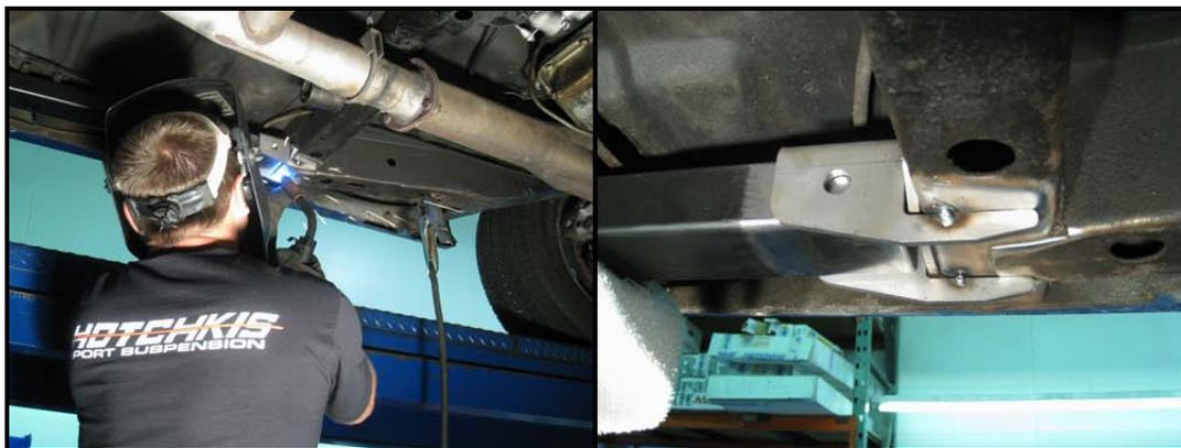
**9. Clean Surface / Weld Mounting Bracket / Install Subframe / Weld Subframe**
