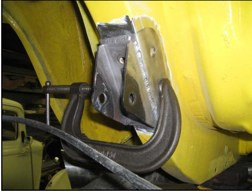
Weld the bracket to the frame rail as shown below.
