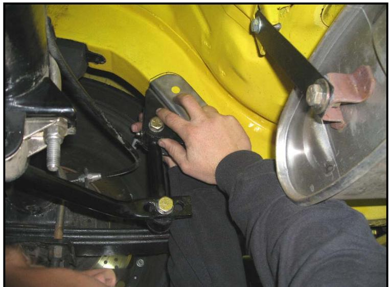
Place the reinforcement bracket onto the frame rail and position the sway bar triangle frame bracket up against the reinforcement bracket. Mark the frame rails outlining the entire bracket including the side holes. Do this for both sides.
