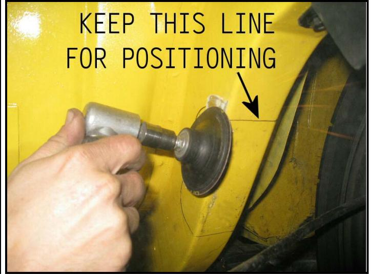
Sand the frame triangle bracket in the sections showed below.
