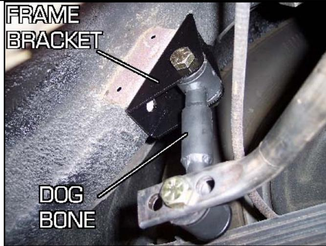
We've noticed on some E-bodies that the distance between the left and right frame rails were 1/2" wider. If the frame bracket does not line up in the center of each frame rail due to the frames having a wider span, then please install the optional spacer between the sway bar and the end link.
