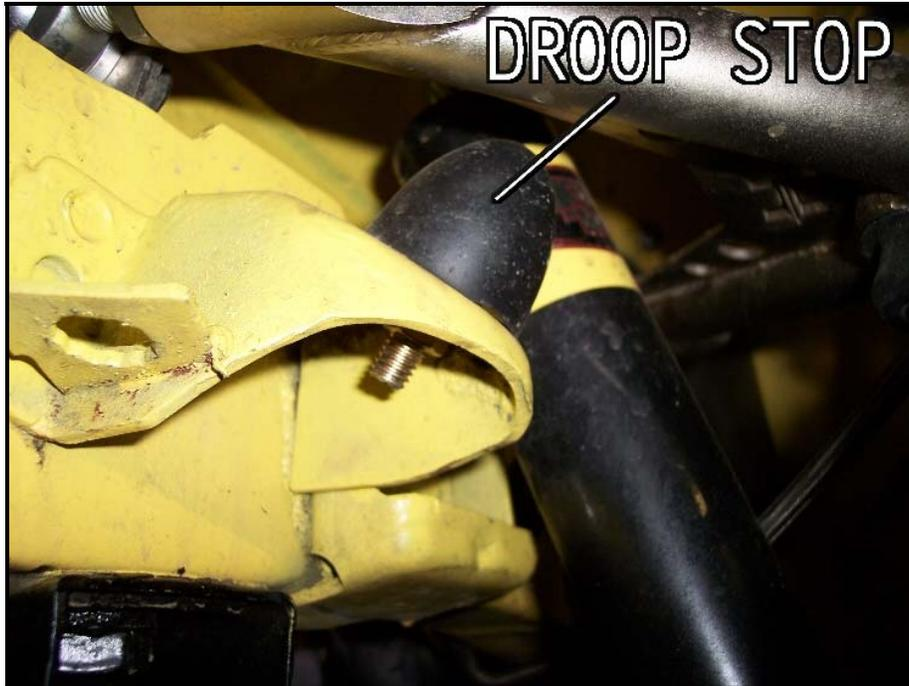
Remove the stock bump stop and install the included Hotchkis "Rectangle" Shaped version.
