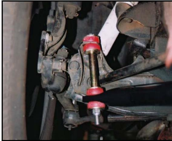
6. Once the end links are attached, install the bushings and brackets to the bar. Make sure to apply the included silicon grease. You will also need to install the new Hotchkis bushing retainer bracket onto the bushing bracket as shown in the picture. Attach the driver and passenger side D-Shaped bushing & bracket and position them as outboard as possible.
