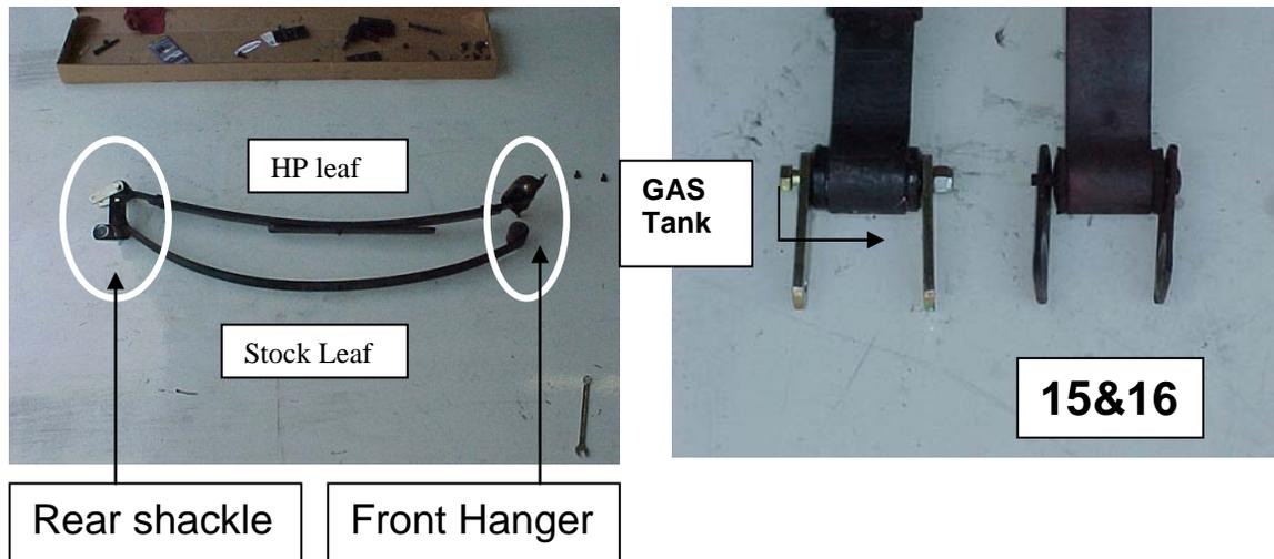
16. Install the leaf springs. You need to set the vehicle on its wheels before you perform the final tightening on the leaf spring eyelet bolts. You must do this so you don't ruin the leaf spring bushings.
