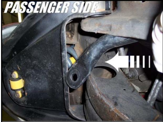
At this point the sway bar will need a little force to get into position. Take your trusty dead blow hammer and hit the anti-roll bar end as shown in the picture below. It won't take too much to pop it into place.
