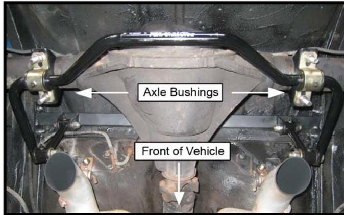
6R. Take a screwdriver and carefully pry up the brake line to allow the U-Bolt to drop down over the axle. (7)
