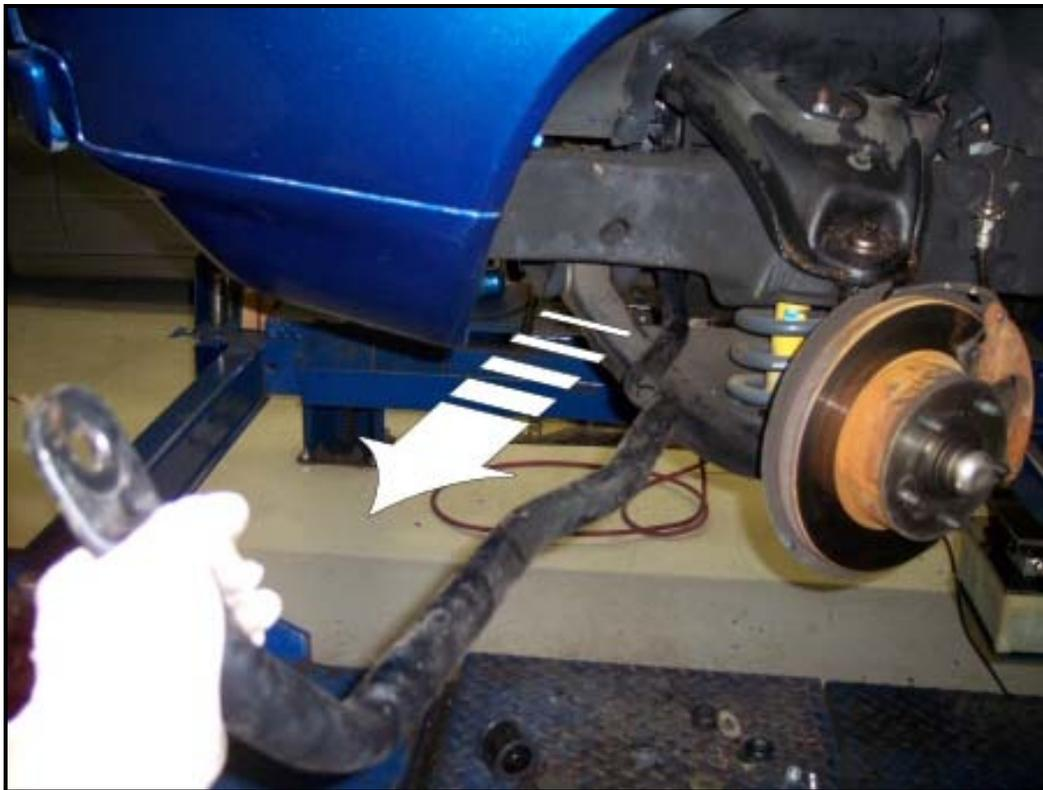
*Installing New Hotchkis Anti-Roll Bar*
