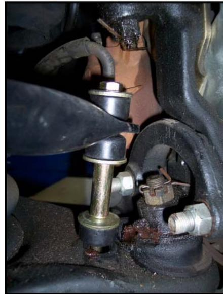
9F. Using the included white silicon grease, lube the inside of the new 1 ¼" front bushings.
