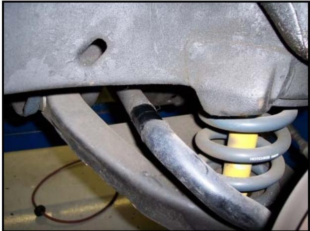
6F. Turn the steering all the way to the LEFT and remove the stock bar through the DRIVER side wheel well. Observe the following pictures for the removal procedure.
