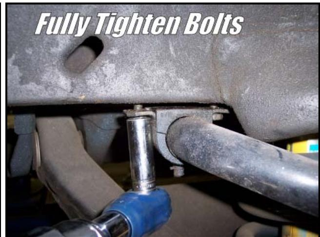
12F. It is best to tighten the endlinks with the suspension at ride height. To achieve this, simply reinstall the wheels and drive the car onto some floor ramps. These can be found at your local auto store. Now, with the car at ride height and on the floor ramps you can crawl underneath the car and fully tighten the endlinks. Tighten the endlinks until the bushings are squeezed just enough that their diameter is just larger than the supporting washer.
