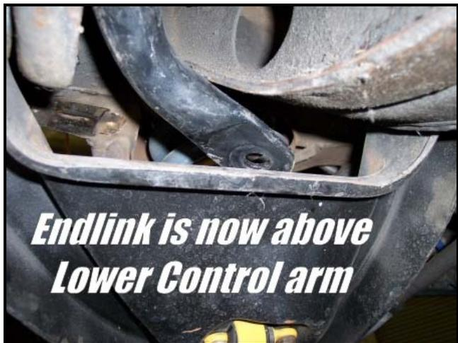
Once the anti-roll bar end is above the lower control arm, you can easily slide it into position.
