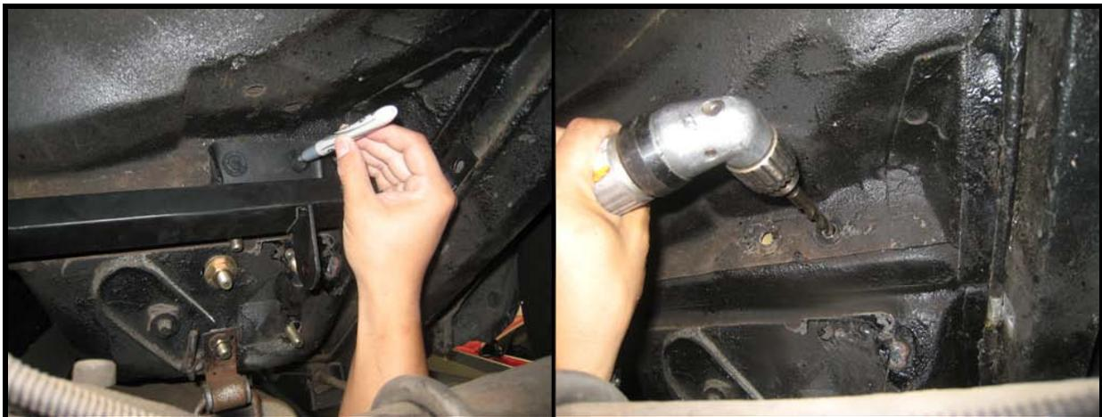
13R. Using the 1718 Hardware kit, pull out the U-Bolts and coat the threading with the Anti-Seize Lubricant.
