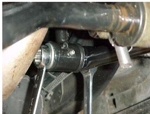
**WARNING:** Check the end link clearance to the bracket hardware. If the hardware contacts the end link it can wear a hole through the end link as the bar rotates in use. You will not be able to install the bar if the stud plate makes contact with the end link.
